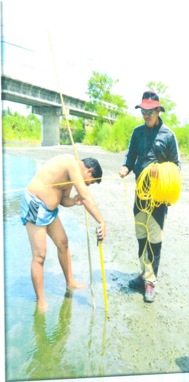
Measurement of water Discharge of Mag-asawang tubig River taken at Mid-section of the river located at Brgy. Pinagsabangan , Naujan. Or. Mdo.
