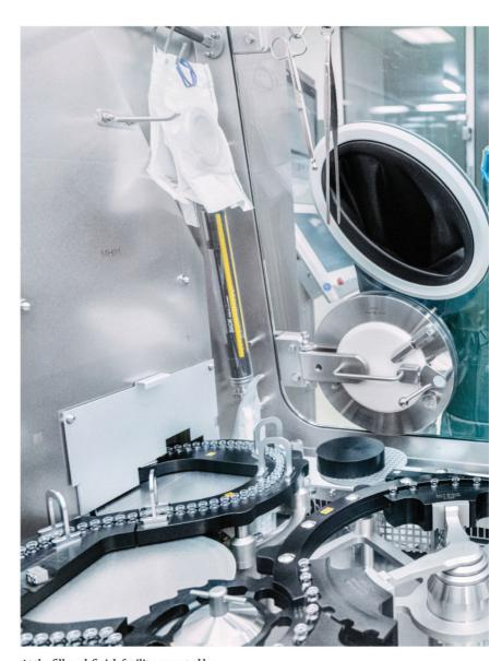
At the fill-and-finish facility operated by Baxter International in Halle, 120 miles north of Marburg, technicians monitor the washing and sterilization of the vials before they are filled with vaccine, then stoppered and sealed
