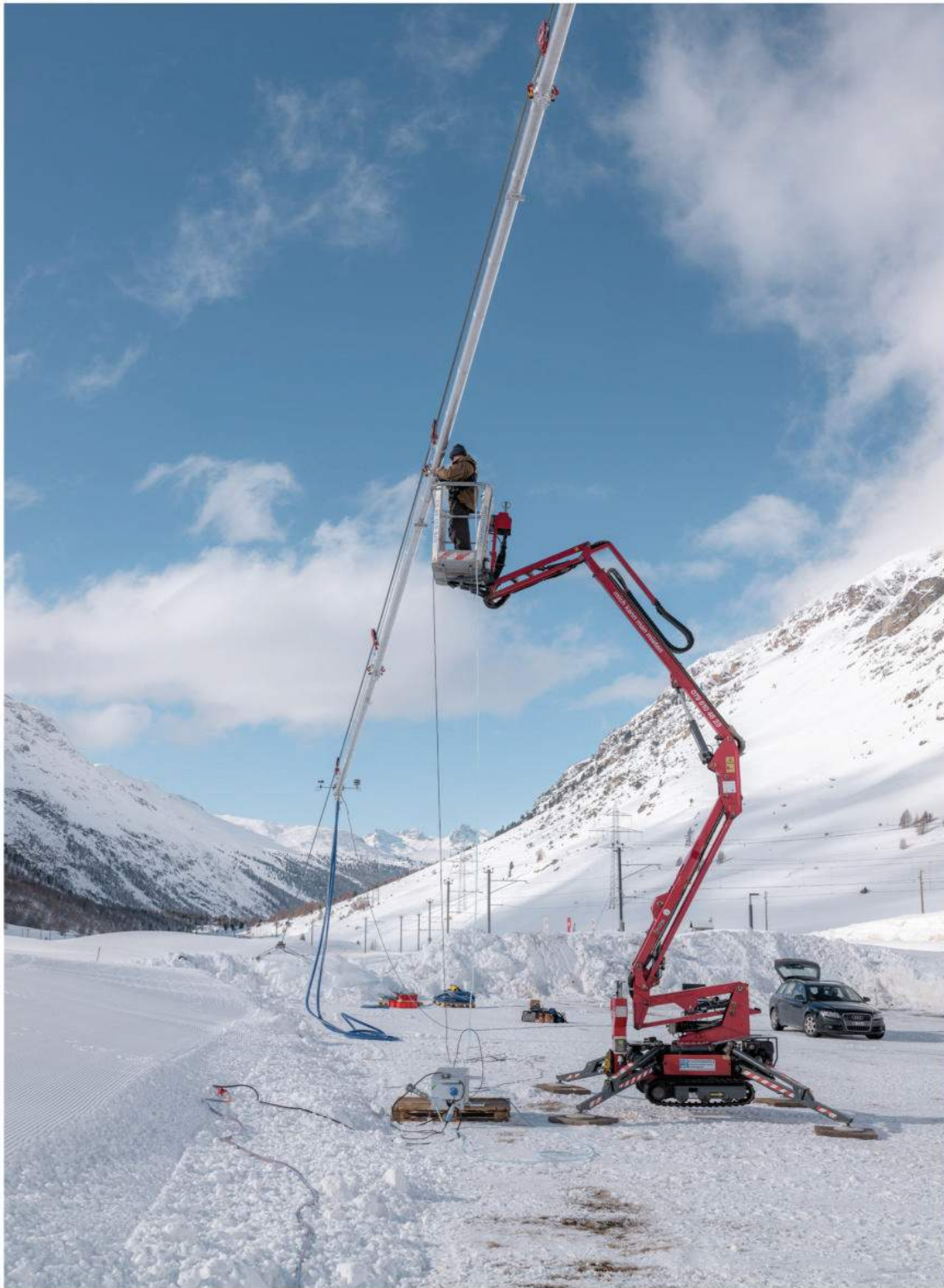
Keller's plan is to recycle glacial meltwater into snow. Here his team tests a prototype of one of the "snow cables" that, hanging over the glacier, would shower it with 30 feet of snow annually.
