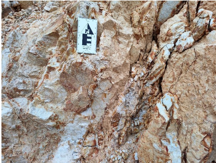
Photo 4. Highly fractured, weathered chert.
