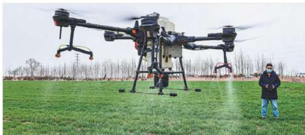
A drone is used to spread pesticide on fields in Hushan town, Rongcheng of Shandong province. LI XINJUN / FOR CHINA DAILY
