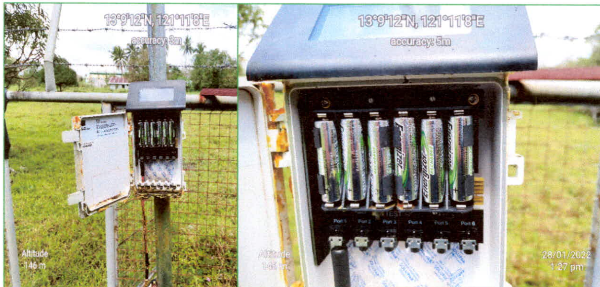
Figures 8: Pictures showing the inside of the data logger of the CTD with the battery compartment showing signs of rust due to the moisture that penetrated the device.
