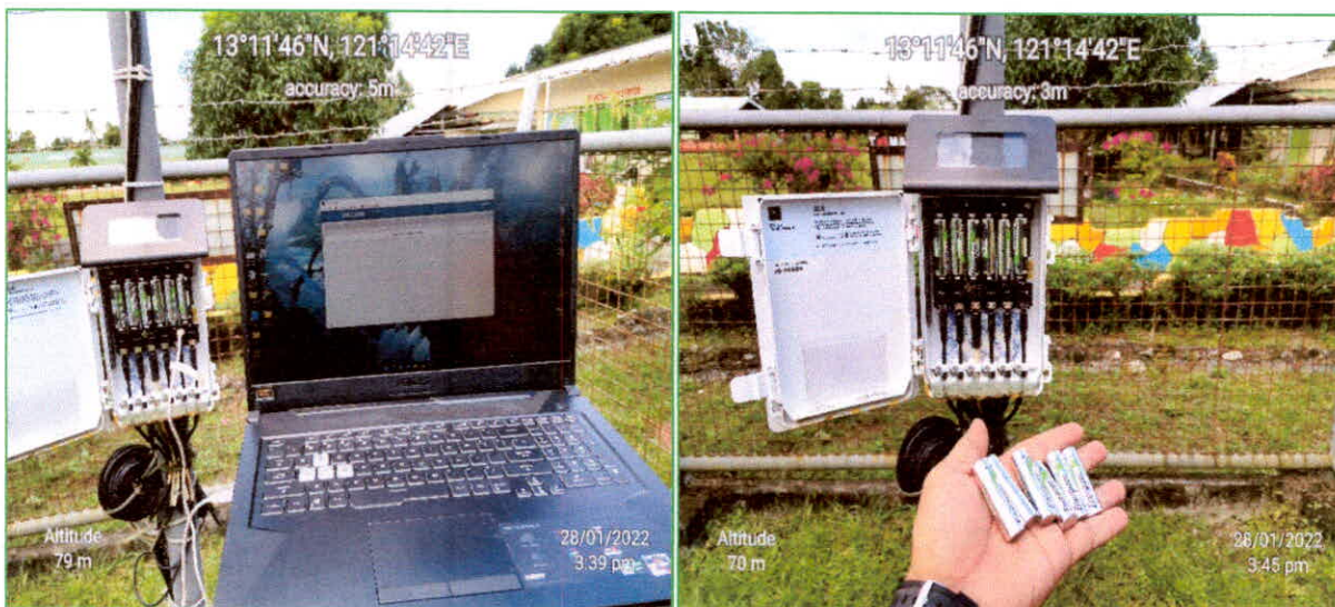
Figures 10: Pictures showing the rechargeable batteries for replacement to the old ones and the manual updating of the firmware of the data logger of the AWS
