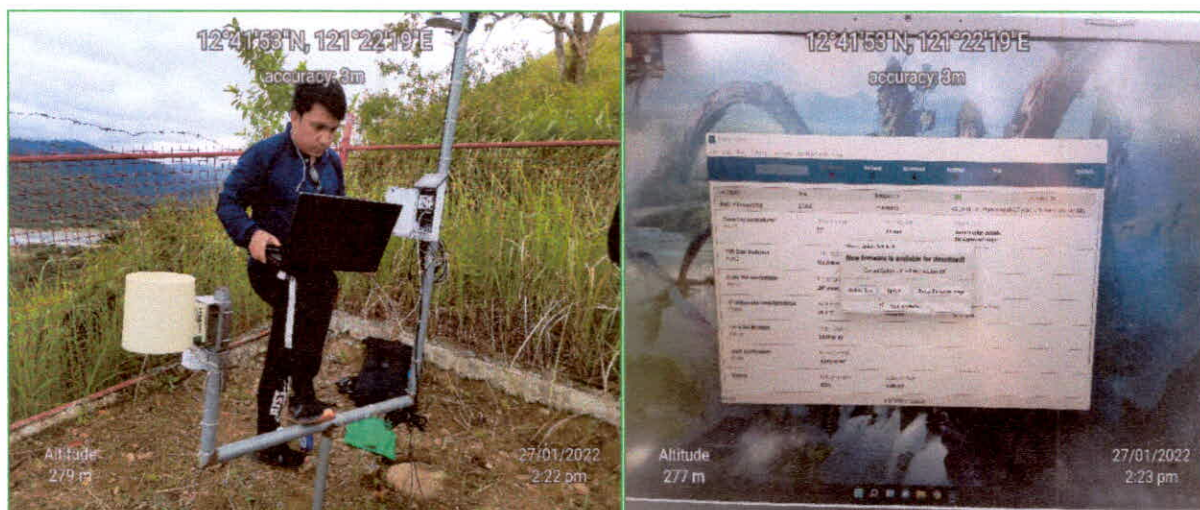
Figures 2: Photos showing the manual updating of the firmware of data logger thru the use of a laptop with updated Zentra Utility app.
