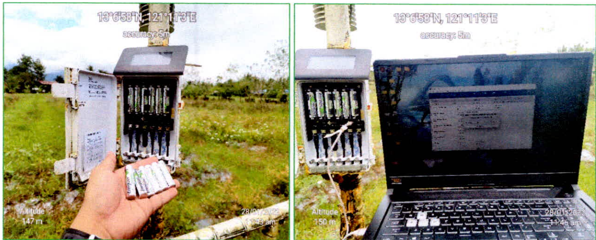
Figures 6: Pictures showing the rechargeable batteries for replacement to the old ones and the manual updating of the firmware of the data logger of the AWS
