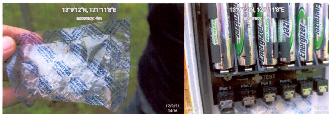
Fig. 2. Rainwater-soaked dessiccant (right) and batteries (left) inside the datalogger of GWMS.
