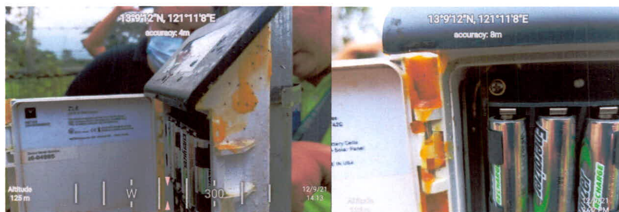
Fig. 3. Ant infestation in the datalogger of GWMS.
