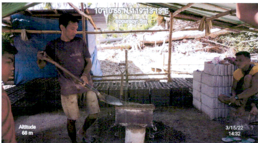
Photo 1. Active production of Hollow Blocks along the Caramay River
