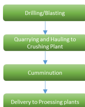
Figure 1. Simplified process flow of RTNMC's quarry and crushing operations
