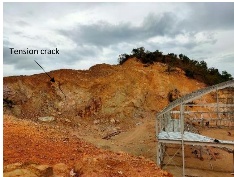
Photo 7. A tension crack was observed on the slope indicating slope
