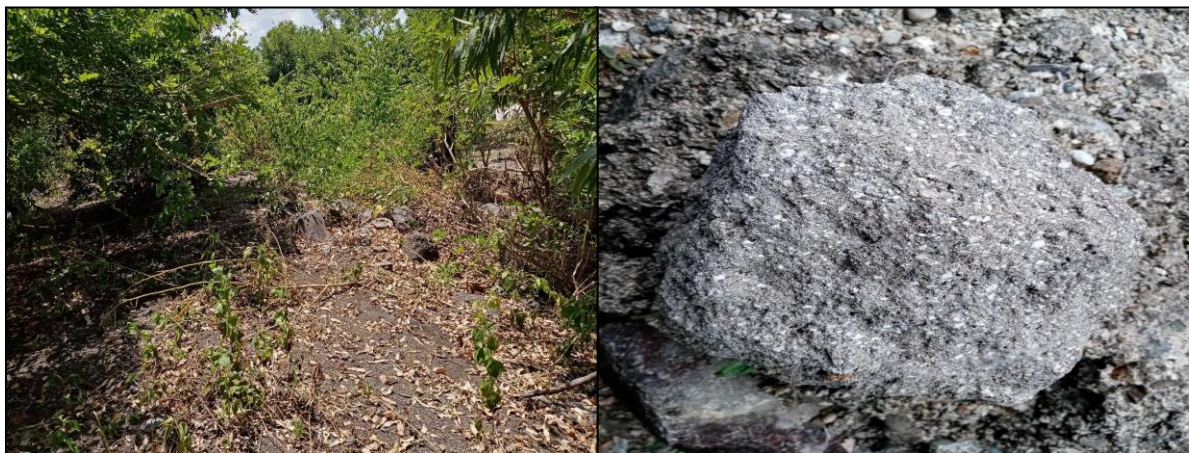
Figure 9. Outcrops of loose cobble to boulder size andesite and tuff along the landfill site
