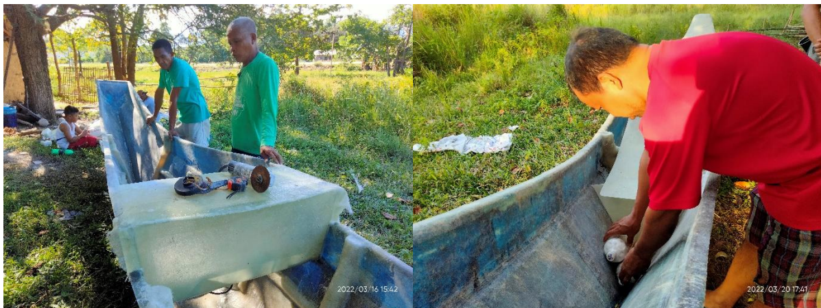
Figure 11. Mold for fabrication of fiberglass boat (left); Mr. Gamad shows how floaters (styrofoam inside pet bottles) are piled in the boat that helps on achieving buoyancy of the boat (right)
