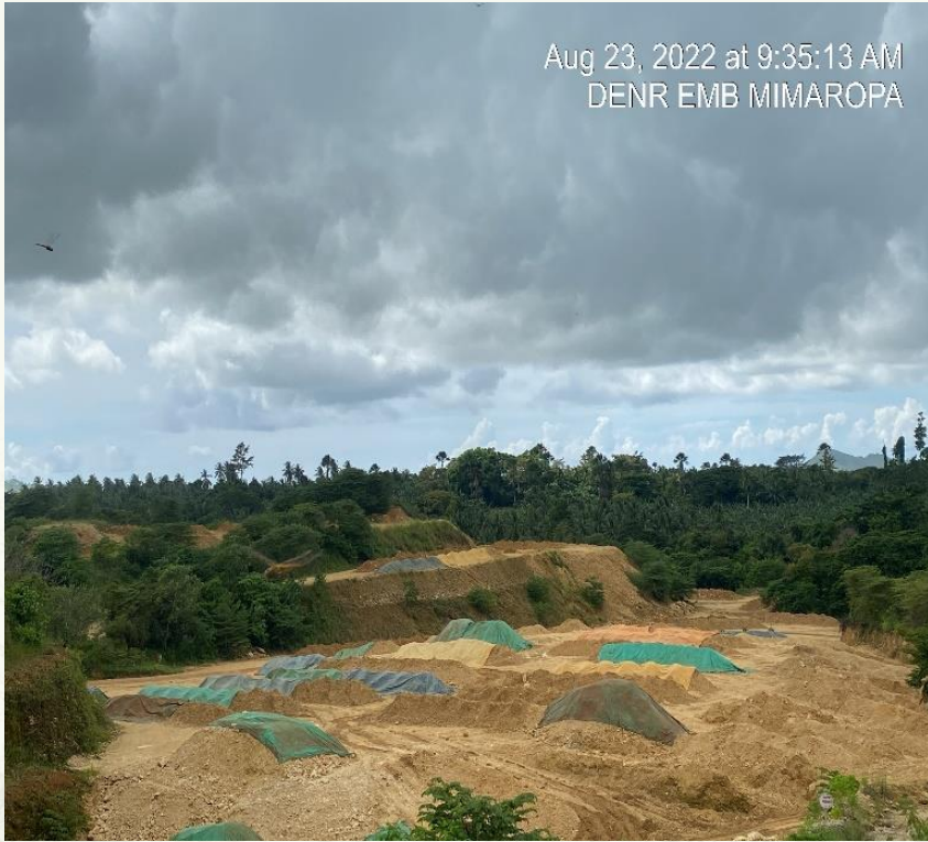
Proper stockpiling of Limestone within the area and on-going recovering of stockpile
