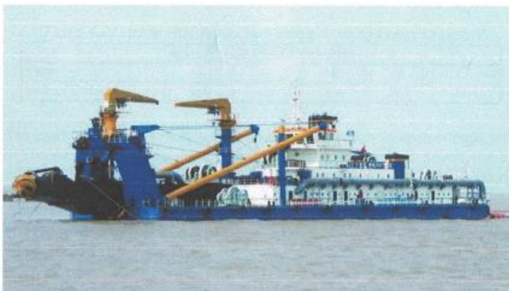
Figure 2. Cutter Suction Dredger
