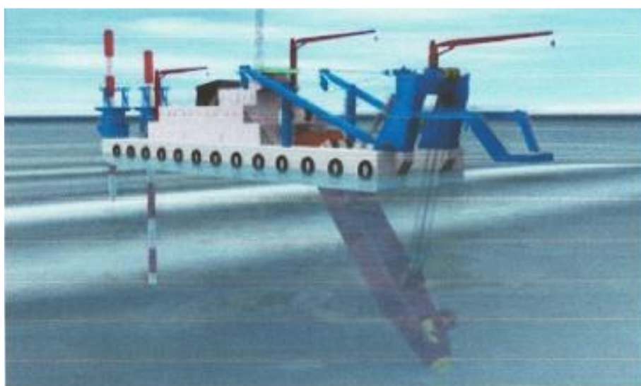
Figure 1-4. Cutter Suction Dredger
