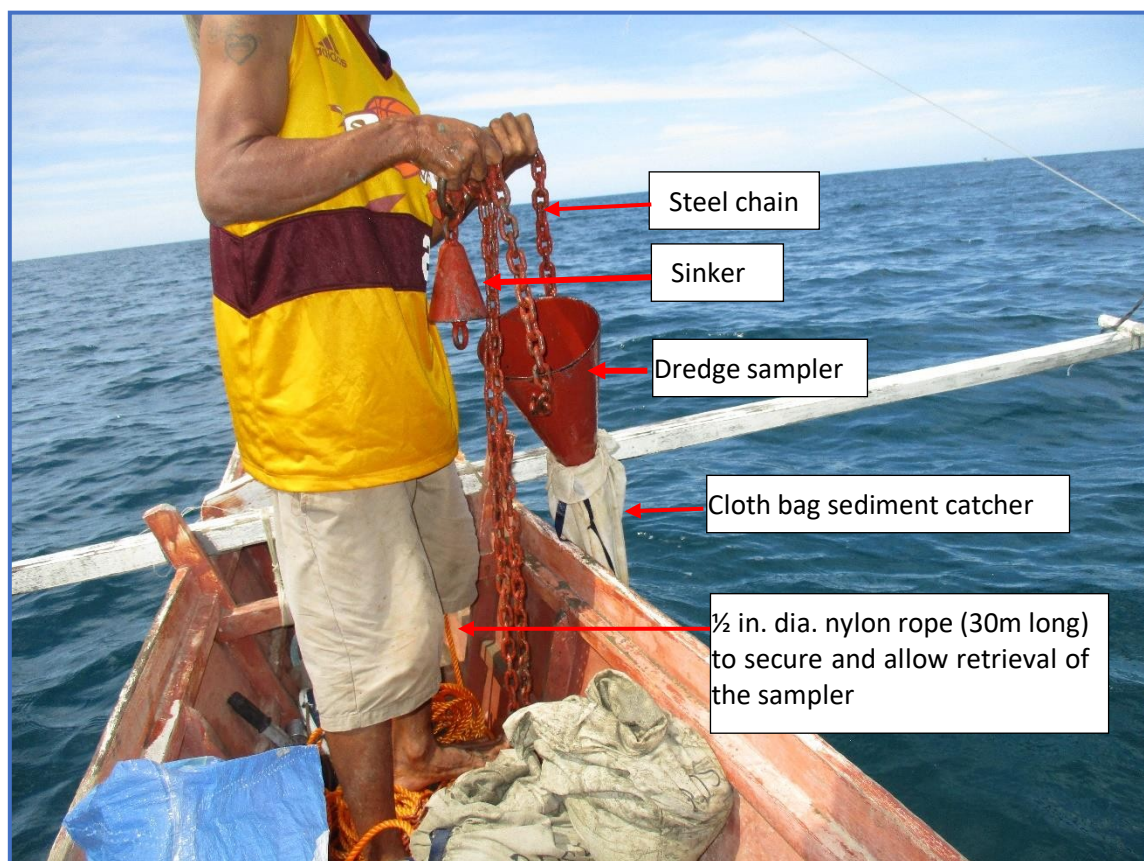
Photo 4. The funnel-shape dredge sampler showing various elements.
