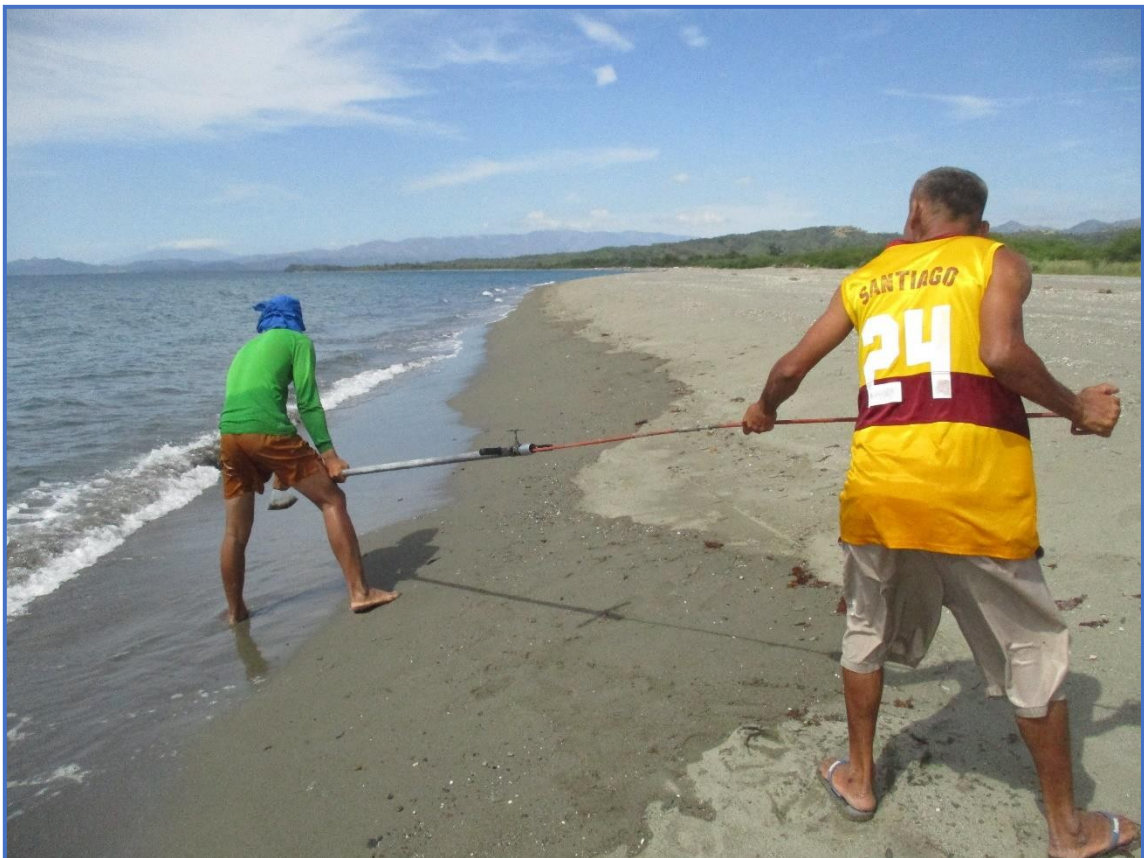
Photo 6. Pushing out the "core" of sand using the sampler's piston
