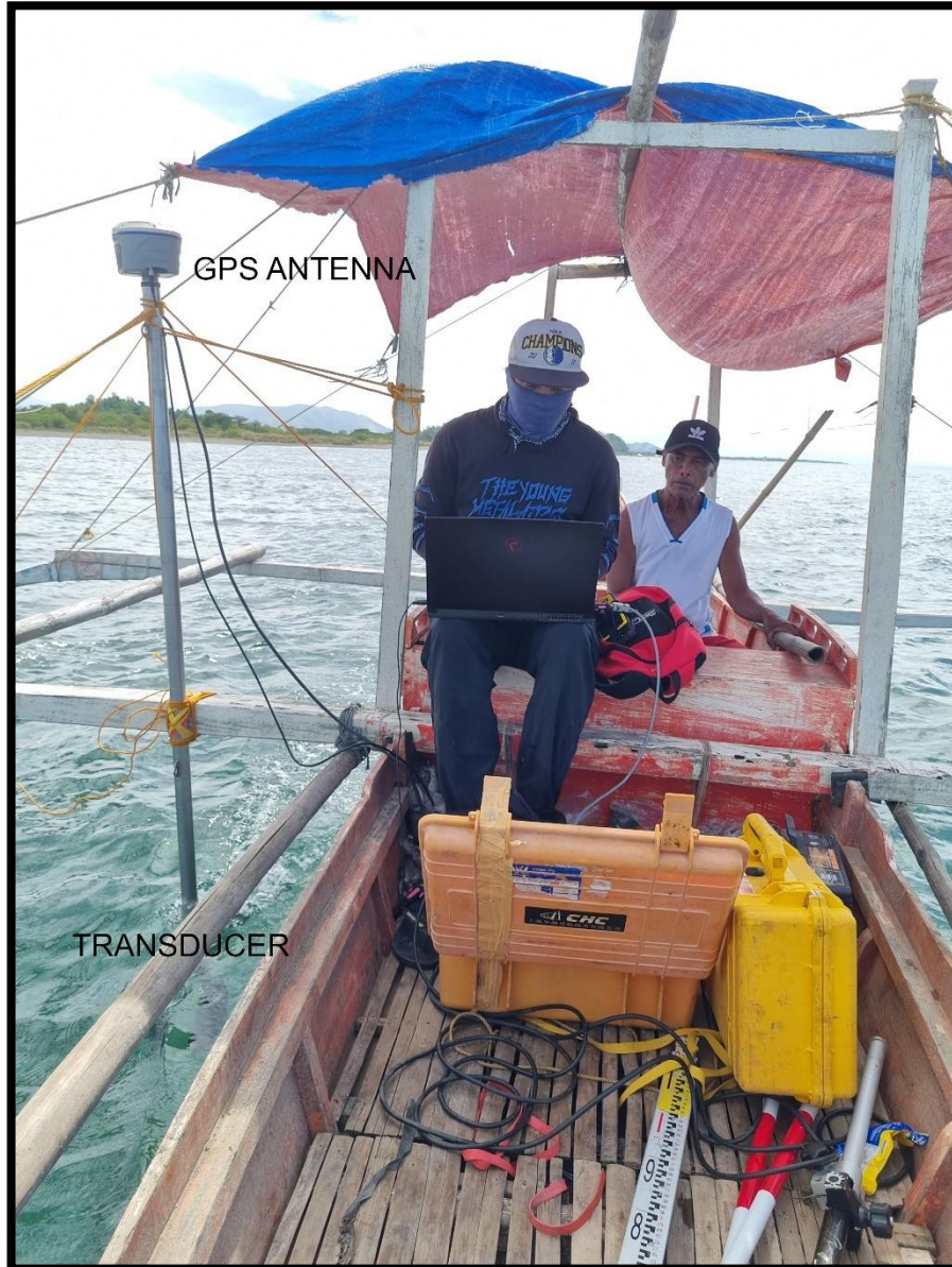
Photo 1 Position of GNSS antenna and transducer in the survey vessel.
