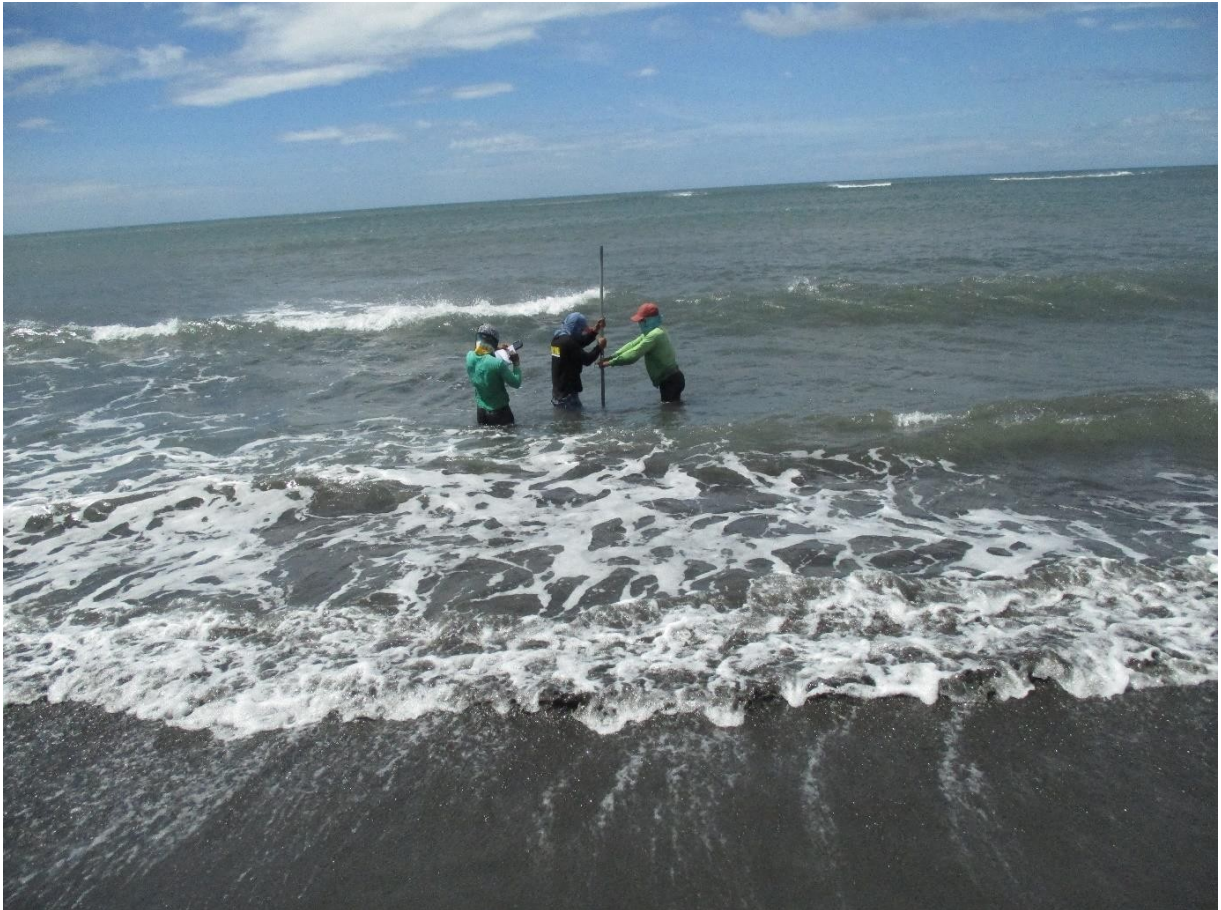
Photo 5. Sand pump sampling at the site of S-SPS-1 [ 12^{\circ}53'45.48''/120^{\circ}46'56.7'' ]
