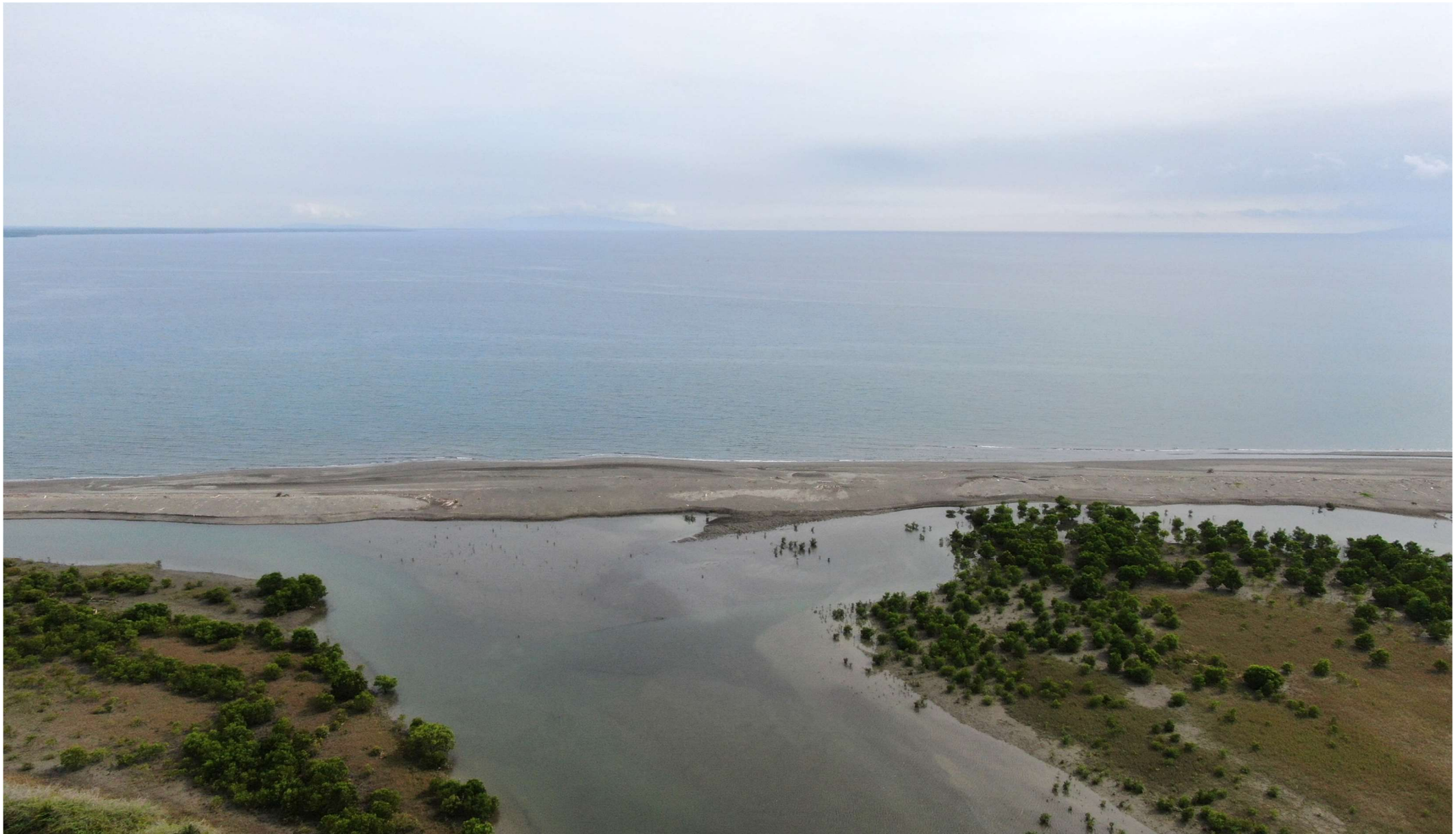
Photo No. 2_Panoramic view of the BONGABONG RIVER using DJI Mavic 2 Zoom Drone showing its distributary stalled by silt materials or sediments.
