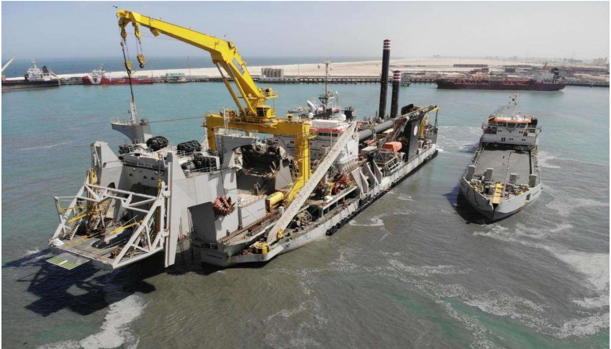
Figure 3_Cutter Suction Dredger and barge.
