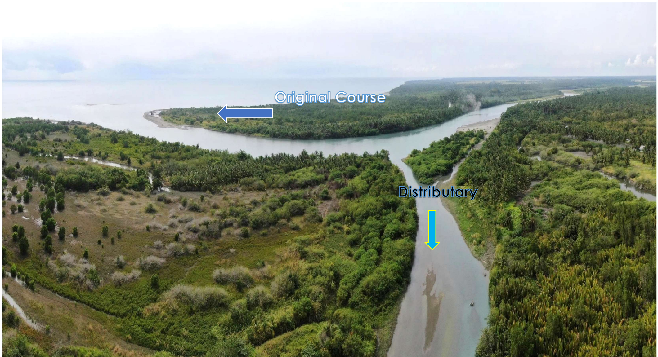
Photo No. 1_Panoramic view of the river delta or the mouth of BONGABONG RIVER using DJI Mavic 2 Zoom Drone. Note that the mouth or the river delta was stalled by silt materials or sediments that prevents the flow of the water including the river run materials to the receiving Tablas Strait causing it to distribute its load to other low-lying area as seen in the photo.
