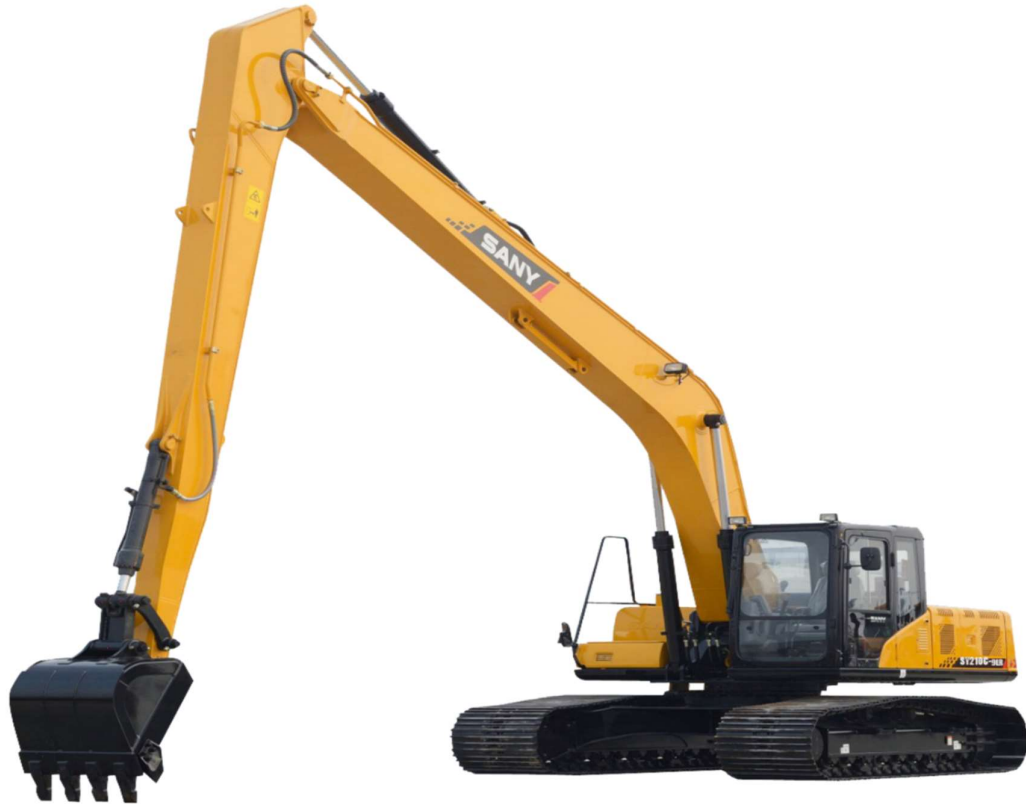
Photo No. 12_Long-arm Excavator with 1.5m 3 capacity bucket for extraction of sand.
