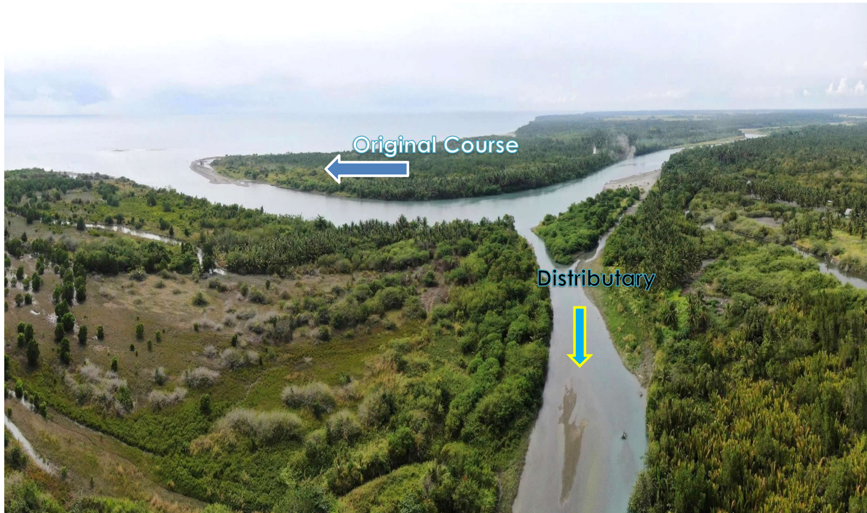
Photo No. 1_Panoramic view of the river delta or the mouth of BONGABONG RIVER using DJI Mavic 2 Zoom Drone. Note that the mouth or the river delta was stalled by silt materials or sediments that prevents the flow of the water including the river run materials to the receiving Tablas Strait causing it to distribute its load to other low-lying area as seen in the photo.
