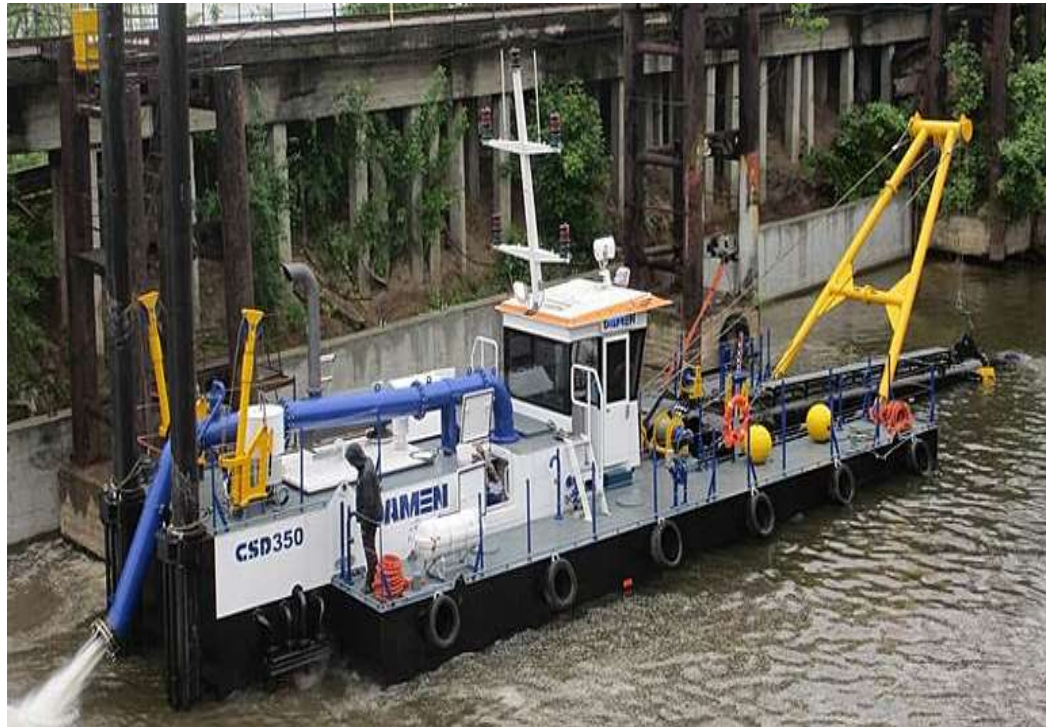
Photo No. 11_This Cutter-Suction Dredger with ID "Damen CSD 350" will be employed initially in the project.
