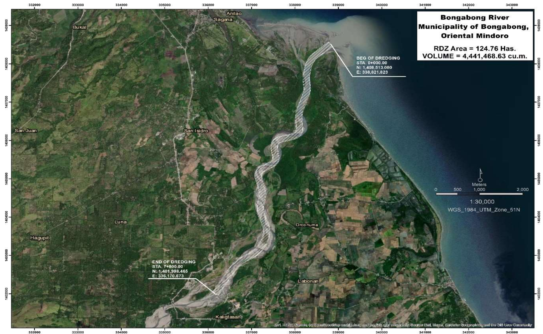
Figure 4_ Satellite Image showing the River Dredging Zone of Bongabong River based on the DPWH Dredging Master Plan.
