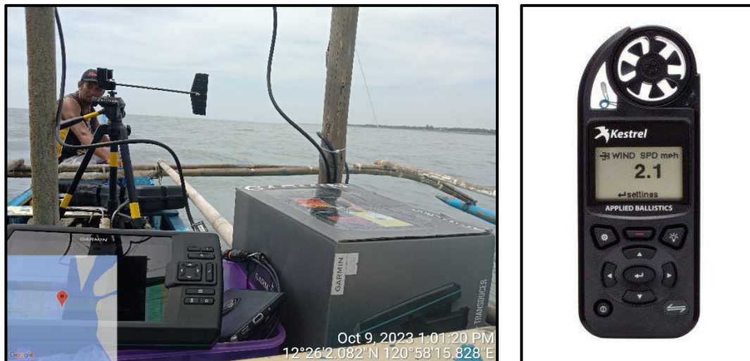
Plate 2.2.2-1. Kestrel NV 4500 Pocket Weather Meter being Used for Data Gathering
