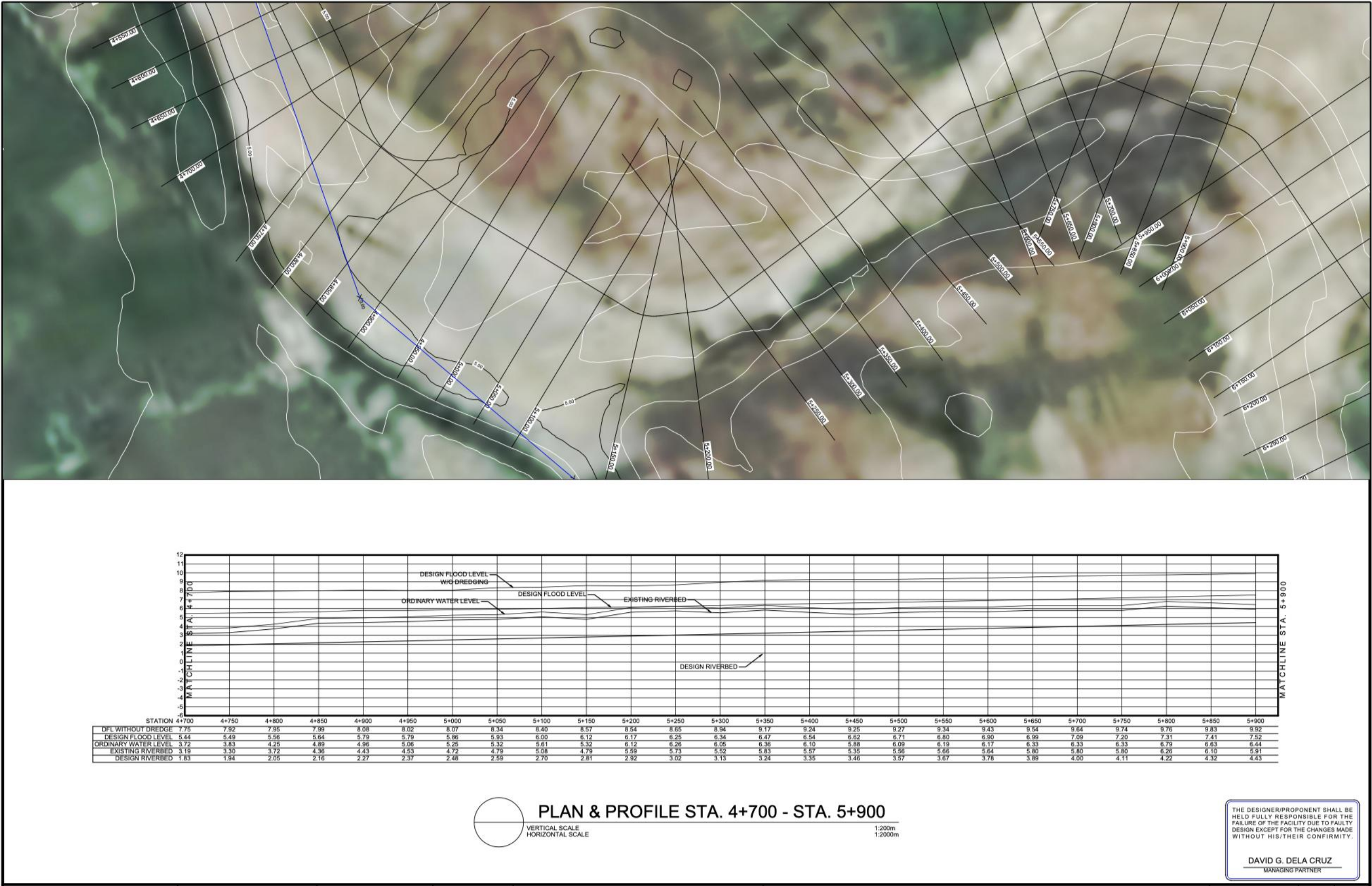
Figure 1-20. Dredging Master Plan and Profile of Project Area (Sta 4+700 to 5+900)
