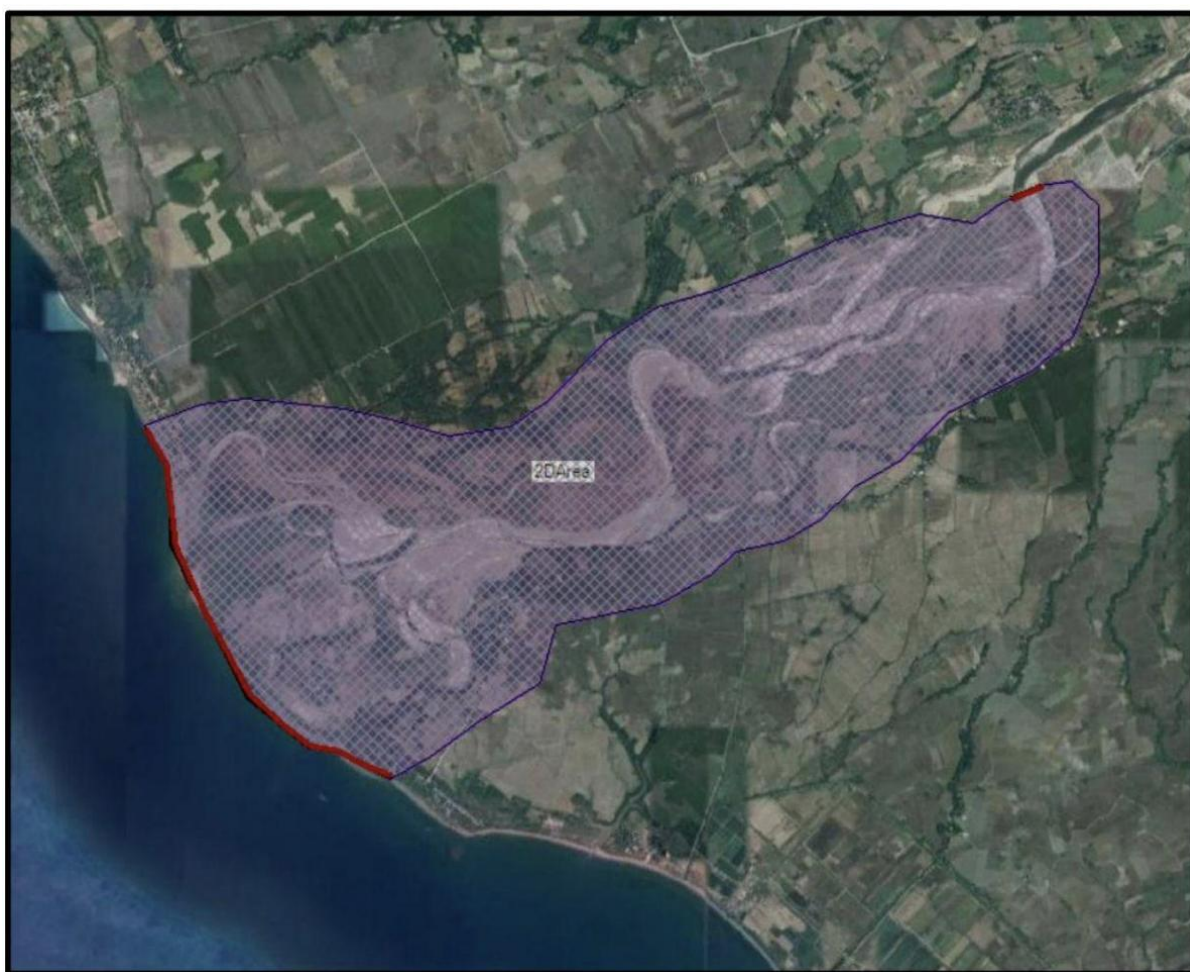
Figure 3-7. Geometric Model for 2D Unsteady Flow Analysis
