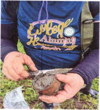
Bulk density sampling using 3cm-core ring
