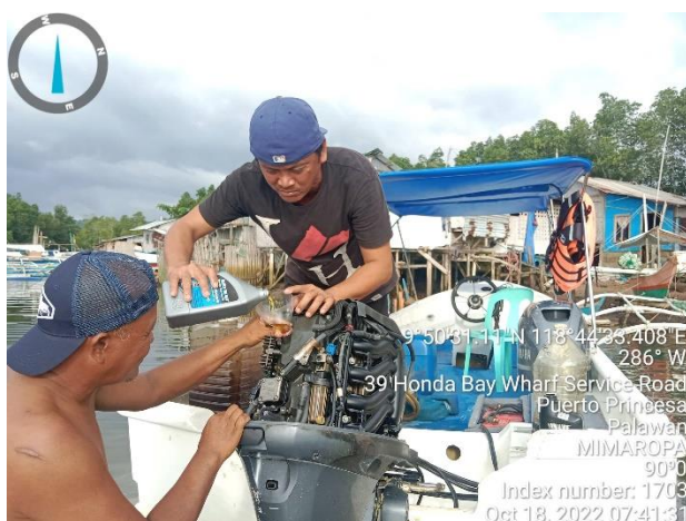
Photos during changing the oil and replacing the oil filter on Yamaha 50 HP
