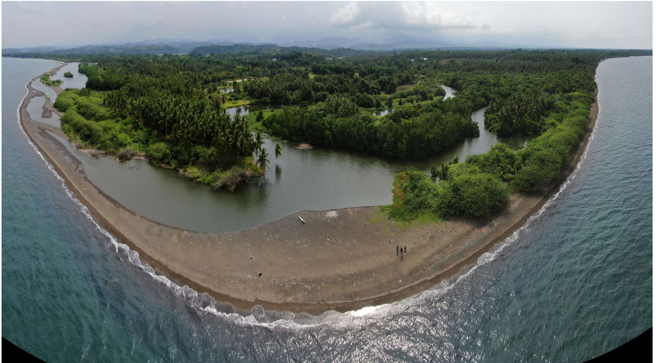
Photo No. 1_Panoramic view of the river delta or the mouth of SUMAGUI RIVER using DJI Mavic 2 Zoom Drone. Note that the mouth or the river delta was stalled by silt materials or sediments that prevents the flow of the water including the river run materials to the receiving Tablas Strait.
