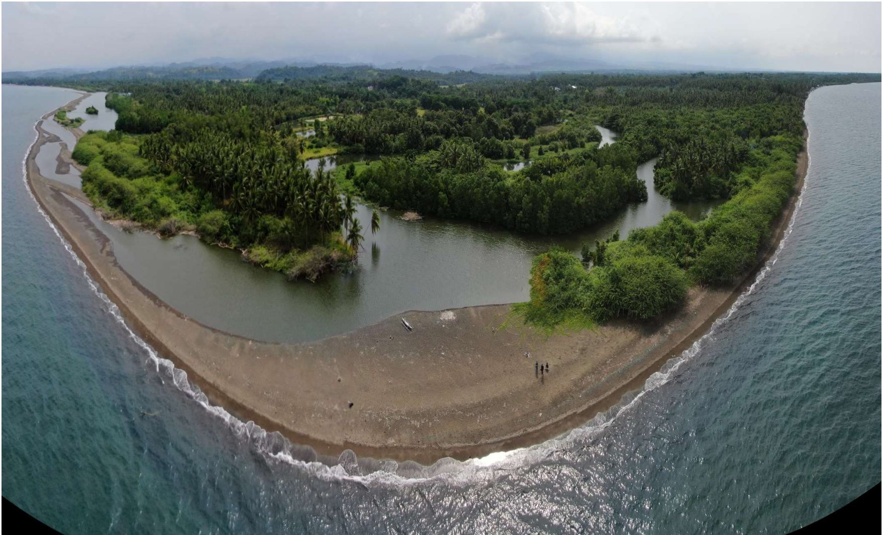
Photo No. 1_Panoramic view of the river delta or the mouth of SUMAGUI RIVER using DJI Mavic 2 Zoom Drone. Note that the mouth or the river delta was stalled by silt materials or sediments that prevents the flow of the water including the river run materials to the receiving Tablas Strait.
