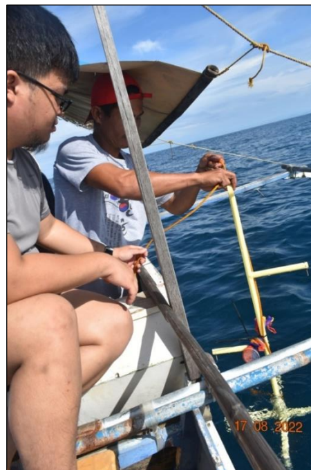
Plate 2.2.22: Deployment of a Camera Mounted on a Metal Frame to Document the Features of the Benthic Substrate
