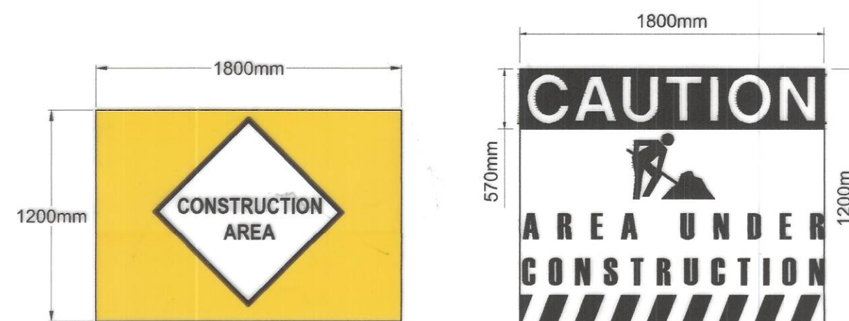
2 26 26 WATERWORKS CONSTRUCTION SIGNAGE
