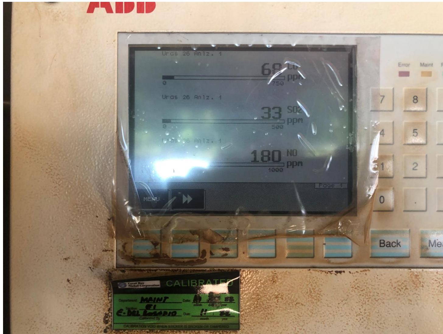
Photo 10. Continuous Emissions Monitoring System of CBNC showing Carbon Monoxide, NO and SO 2 readings that are way below the DENR standards during the MMT monitoring.
