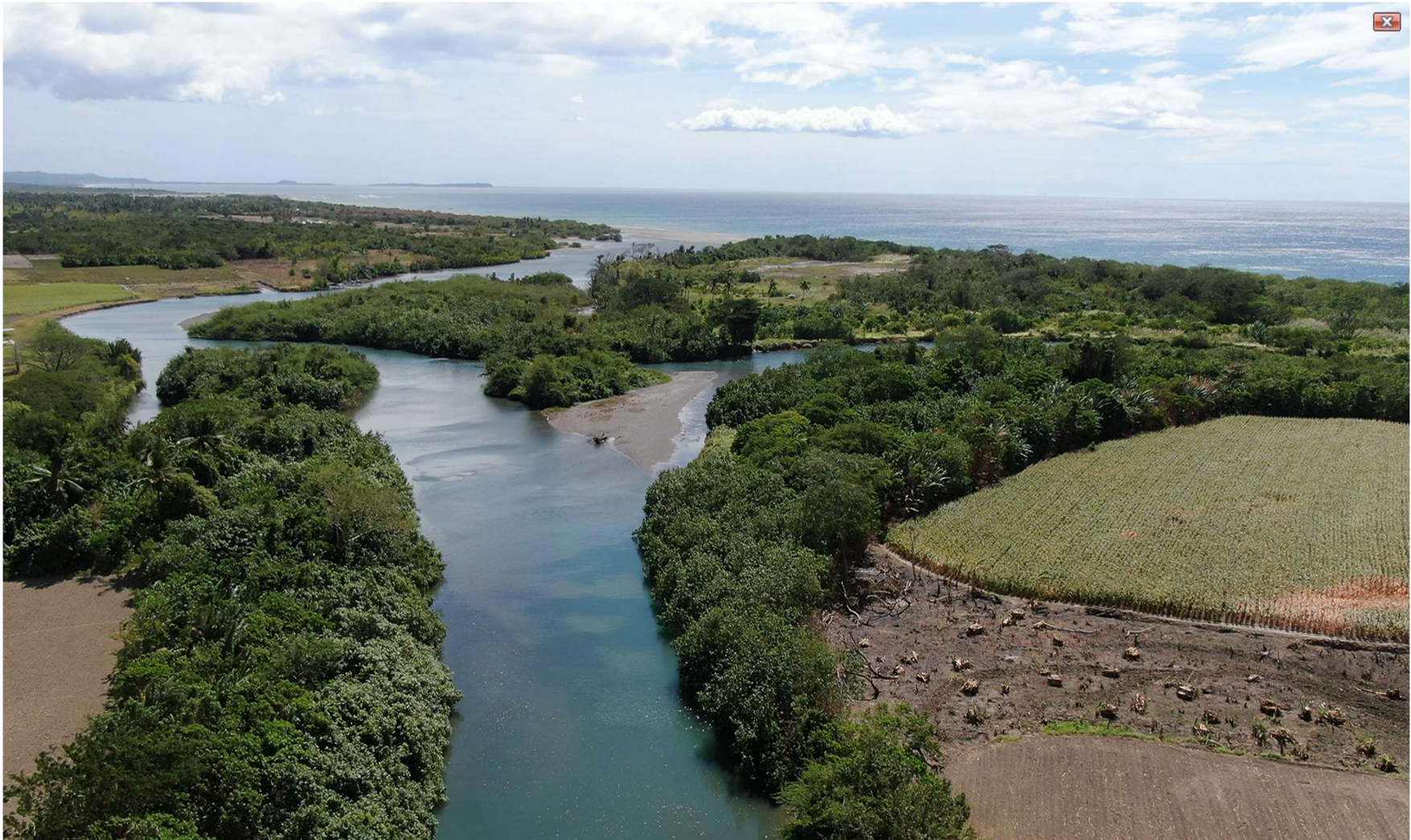
Photo No. 2_Panoramic view of the BACLARAN RIVER using DJI Mavic 2 Zoom Drone showing distributary stream to the right joining Barahan River due to the opening or the mouth of Baclaran River were heavily silted therefore water will find another way to empty its load to Mindoro Strait.
