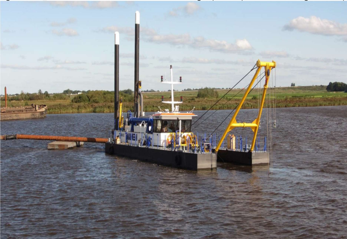
Figure No. 5_This Cutter-Suction Dredger with ID "Damen CSD 450" will be employed initially in the project.
