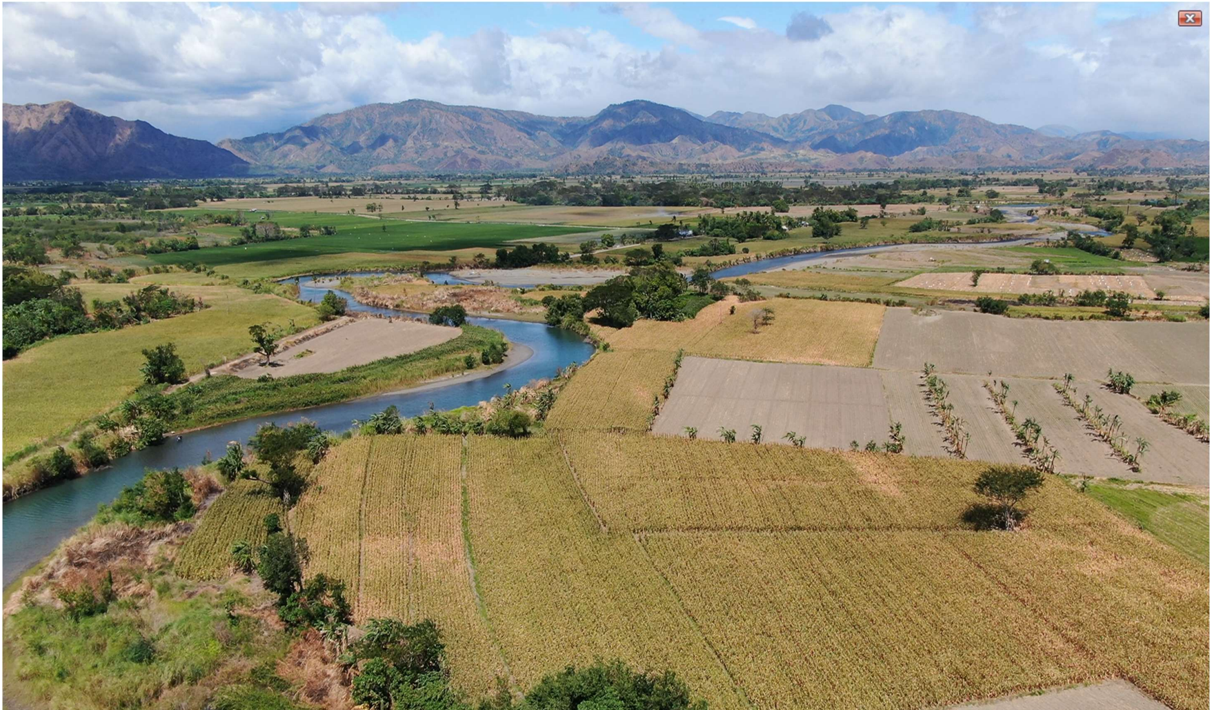
Photo No. 3_Panoramic view showing that crops such as corn and onion were planted to the large portion of the original path of BACLARAN RIVER creating diversion of water to low lying parts of the river system that causes flooding and erosion.
