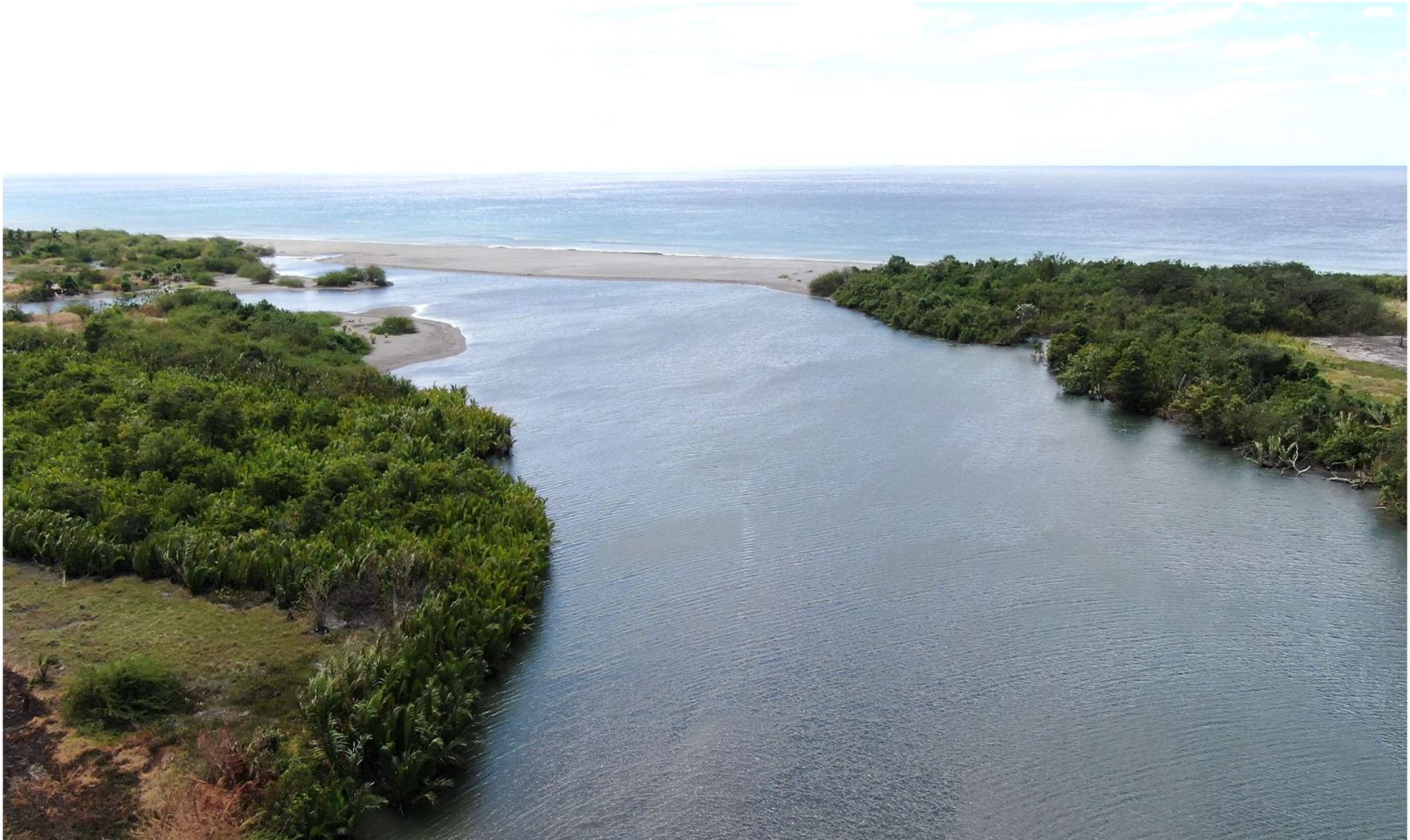
Photo No. 1_Panoramic view of the river delta or the mouth of BACLARAN RIVER using DJI Mavic 2 Zoom Drone. Note that the mouth or the river delta was stalled by silt materials or sediments that prevents the flow of the water including the river run materials to the receiving Mindoro Strait.
