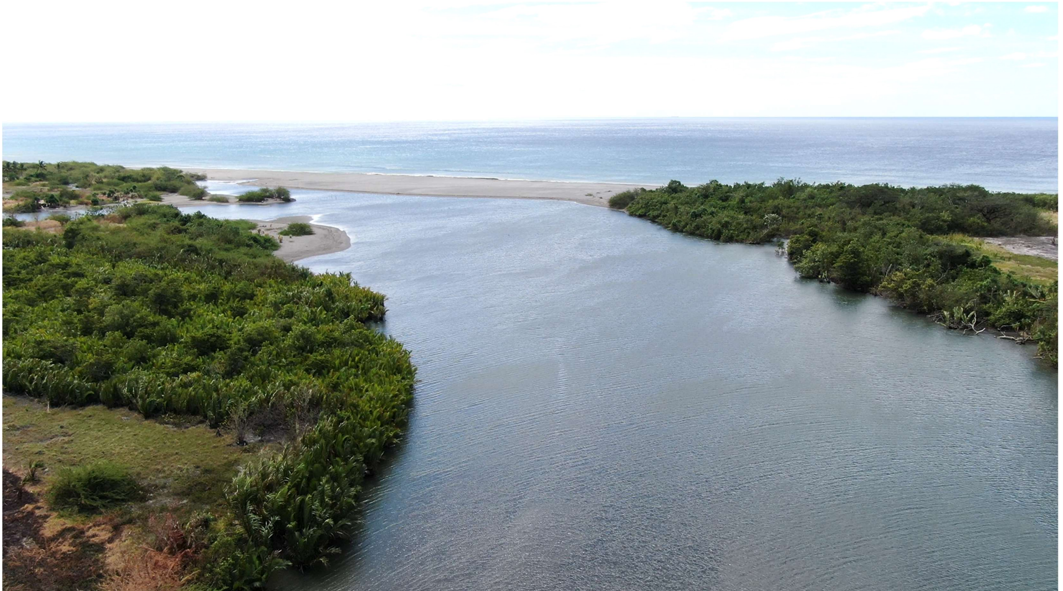
Photo No. 1_Panoramic view of the river delta or the mouth of BACLARAN RIVER using DJI Mavic 2 Zoom Drone. Note that the mouth or the river delta was stalled by silt materials or sediments that prevents the flow of the water including the river run materials to the receiving Mindoro Strait.
