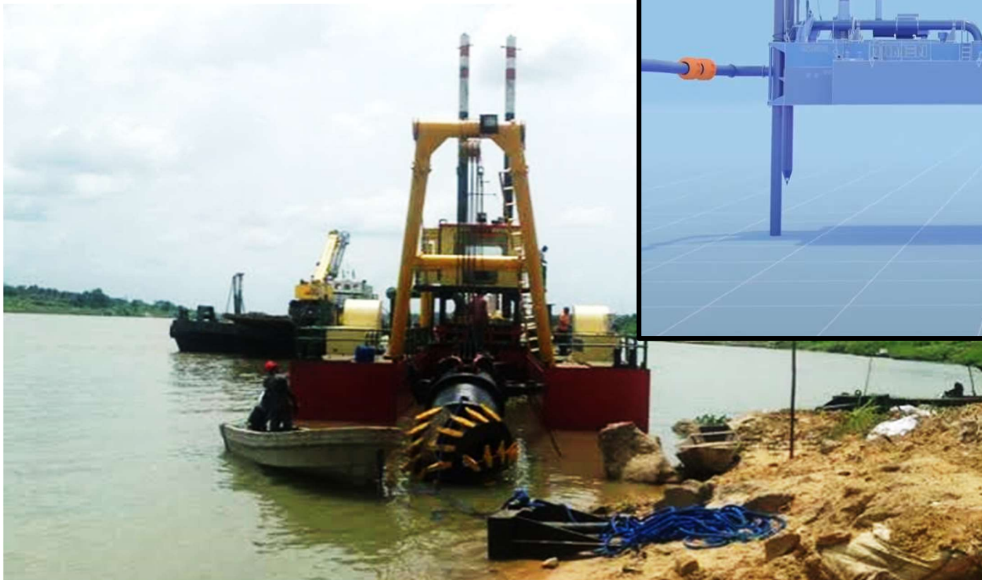
Figure 2_Cutter Suction Dredger – Damen CSD 450, showing 2 spuds to position the dredger steadily.
