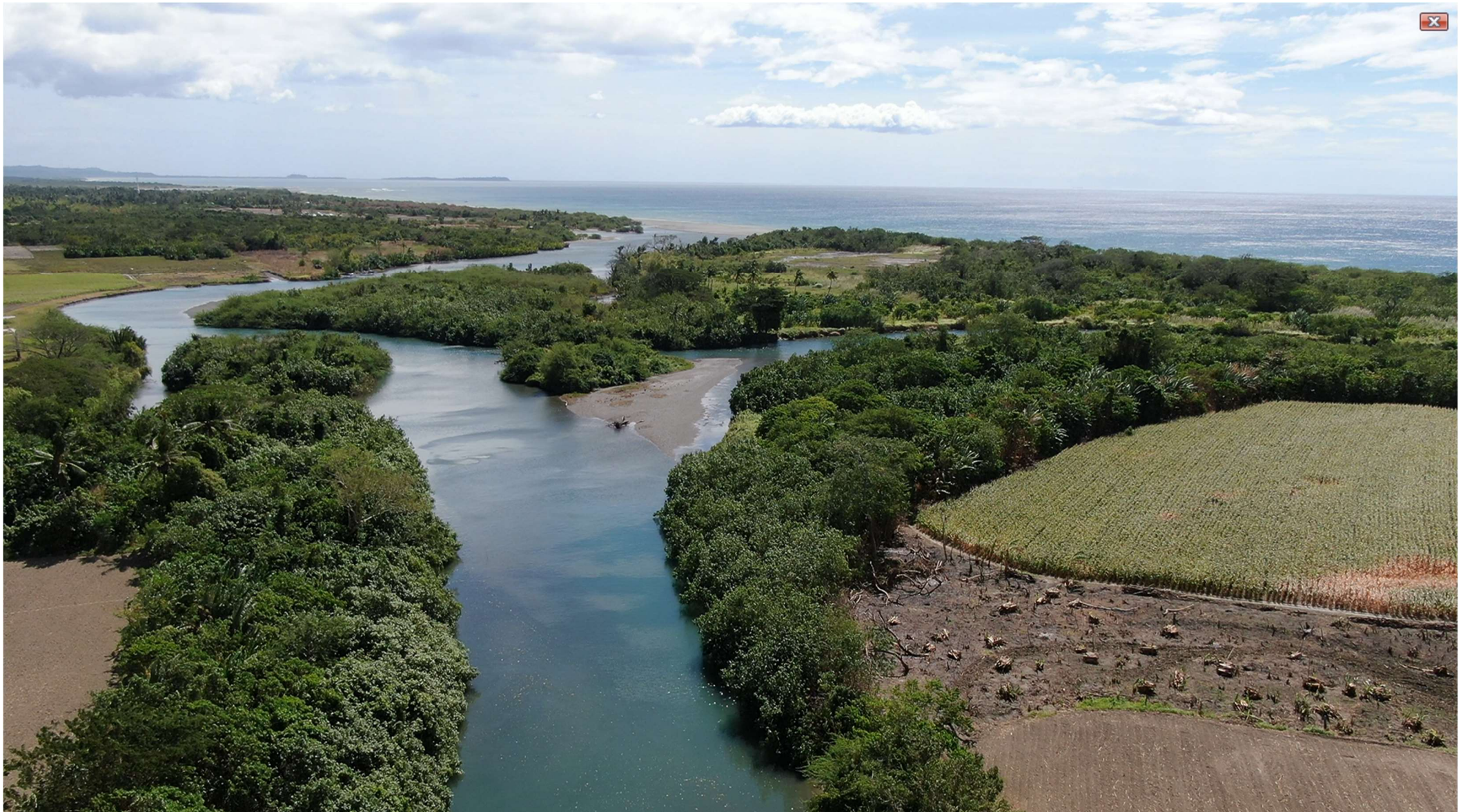
Photo No. 2_Panoramic view of the BACLARAN RIVER using DJI Mavic 2 Zoom Drone showing distributary stream to the right joining Barahan River due to the opening or the mouth of Baclaran River were heavily silted therefore water will find another way to empty its load to Mindoro Strait.
