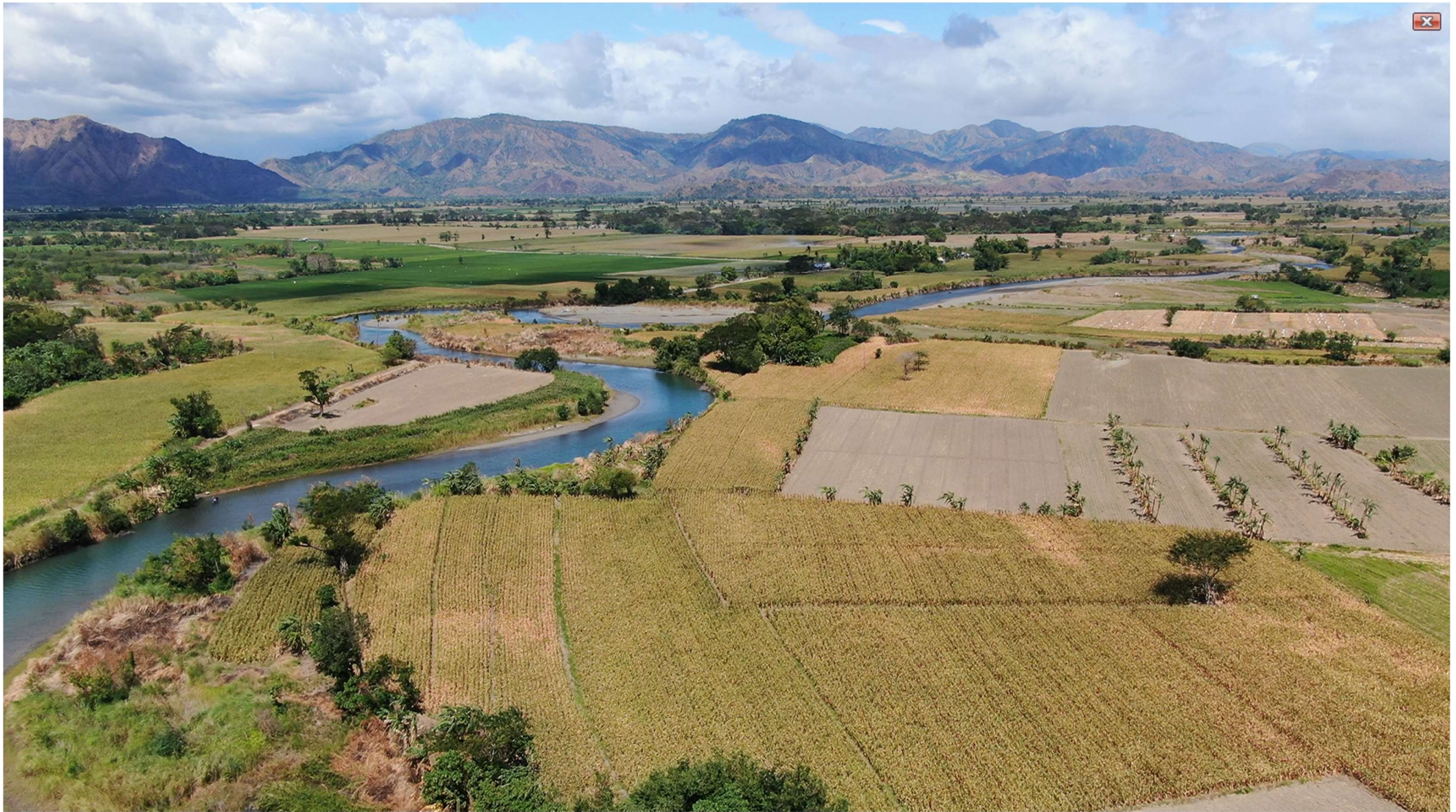
Photo No. 3_Panoramic view showing that crops such as corn and onion were planted to the large portion of the original path of BACLARAN RIVER creating diversion of water to low lying parts of the river system that causes flooding and erosion.
