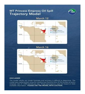
The recent simulation focusing on the area of the tanker's location for March 10 to 16 shows that with continuous seepage of oil, most of the oil will end up along Naujan coast and Pola Bay. However, due to the weakening Amihan, some of the oil may flow northwards towards the Verde Island Passage by March 16, affecting coastal areas of Calapan, Verde Island, and some parts of Batangas.
