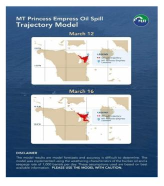
The recent simulation focusing on the area of the tanker's location for March 10 to 16 shows that with continuous seepage of oil, most of the oil will end up along Naujan coast and Pola Bay. However, due to the weakening Amihan, some of the oil may flow northwards towards the Verde Island Passage by March 16, affecting coastal areas of Calapan, Verde Island, and some parts of Batangas.
