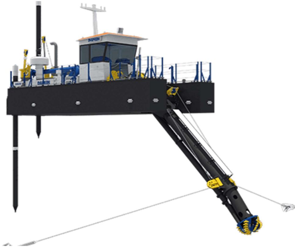
Figure 8_Side View of the Damen CSD 250, showing 2 spuds to position the dredger steadily.
