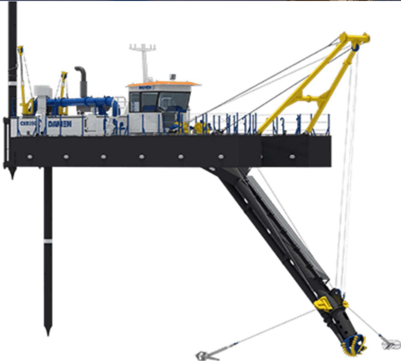
Figure 12 This Cutter-Suction Dredger with ID "Damen CSD 250" will be employed initially in the project. Side View of the Damen CSD 250, showing 2 spuds to position the dredger steadily.
