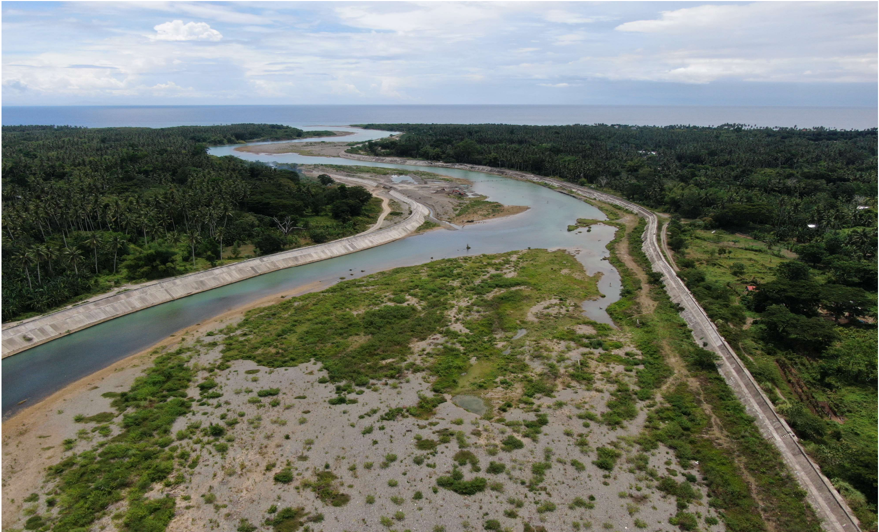
Plate 2 Panoramic view of the BOAC RIVER using DJI Mavic 2 Zoom Drone showing the accumulation of sediments preventing the water and other river-run materials to smoothly flow to Tablas Strait /Tayabas Bay. Riverbanks are protected with concrete dike to prevent overflow / flooding.
