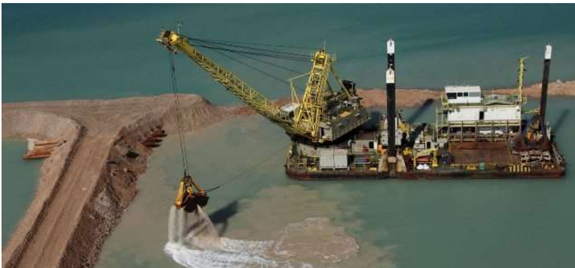
Figure 10 _Van Loon Maritime Services B.V. Grab Dredger with 5-8m 3 clamshell attached to line with dredging depth of 20 meters max (on spuds).
