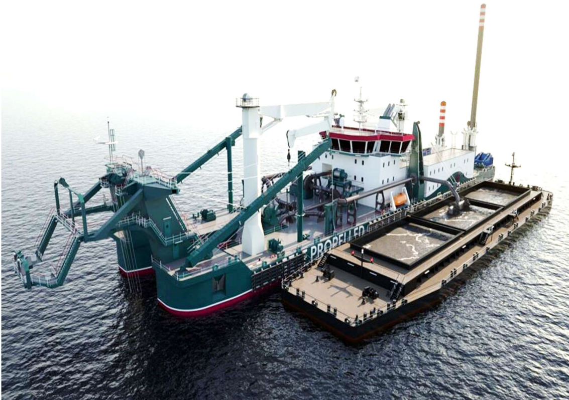
Figure 14 _Loading of Dredged Materials to Floating Hopper Barge.
