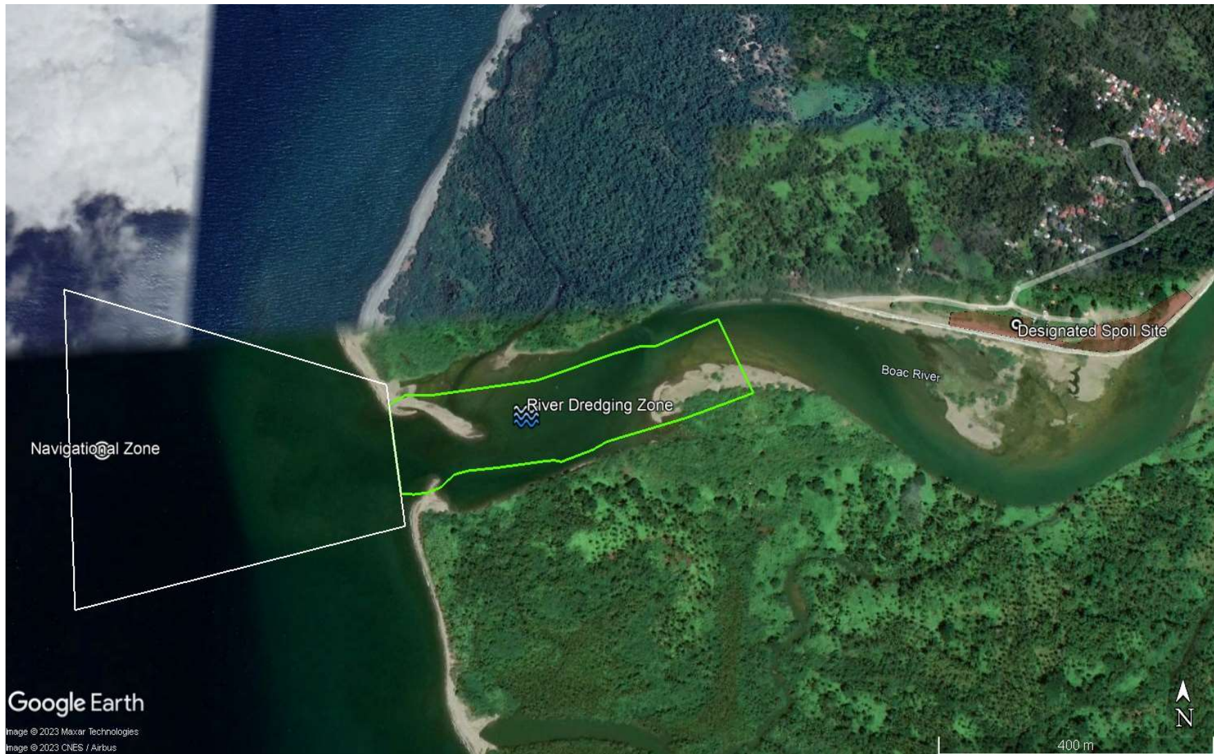
Figure 16 _Satellite image showing the River Dredging Zone, Dredging Navigational Zone and Designated Spoil Site / Area .
