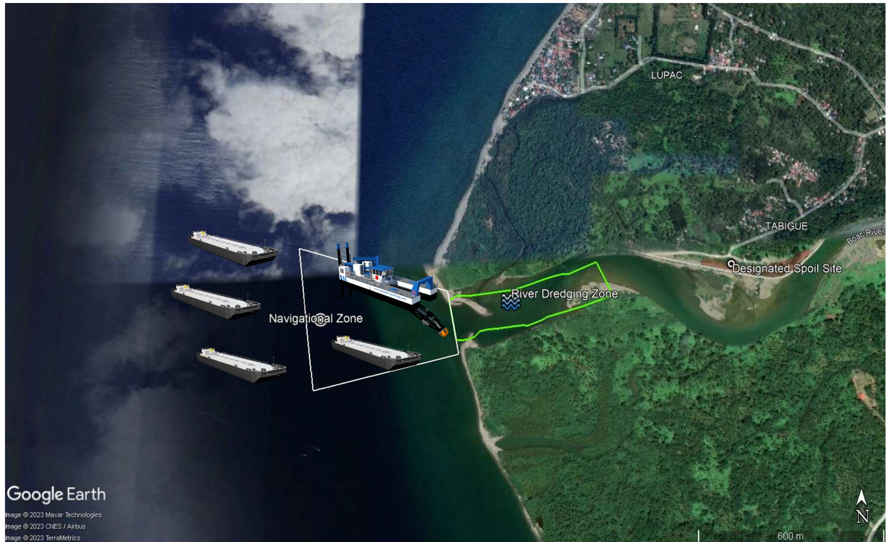
Figure 18 Operation using Cutter-Suction Dredger and immediately transfer to the floating hopper barges and/or sand carrier vessel.
