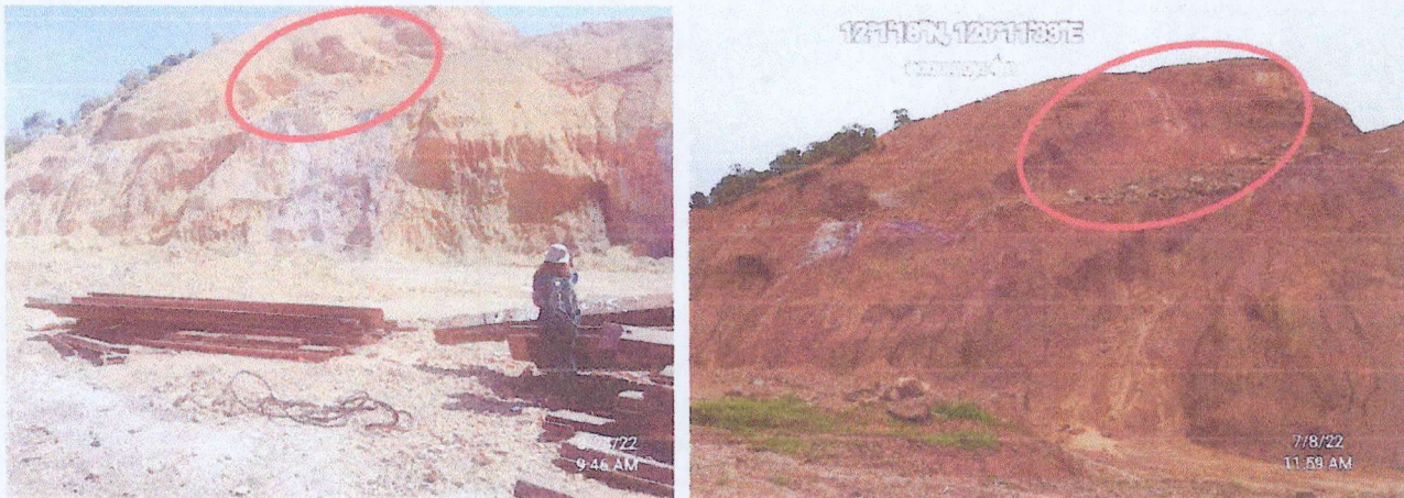
Figure 2. Comparison of the morphology of the area. The image on the left was taken in March whereas the image on the right was taken in July. Encircled is the area where evidence of mass movement was observed.
