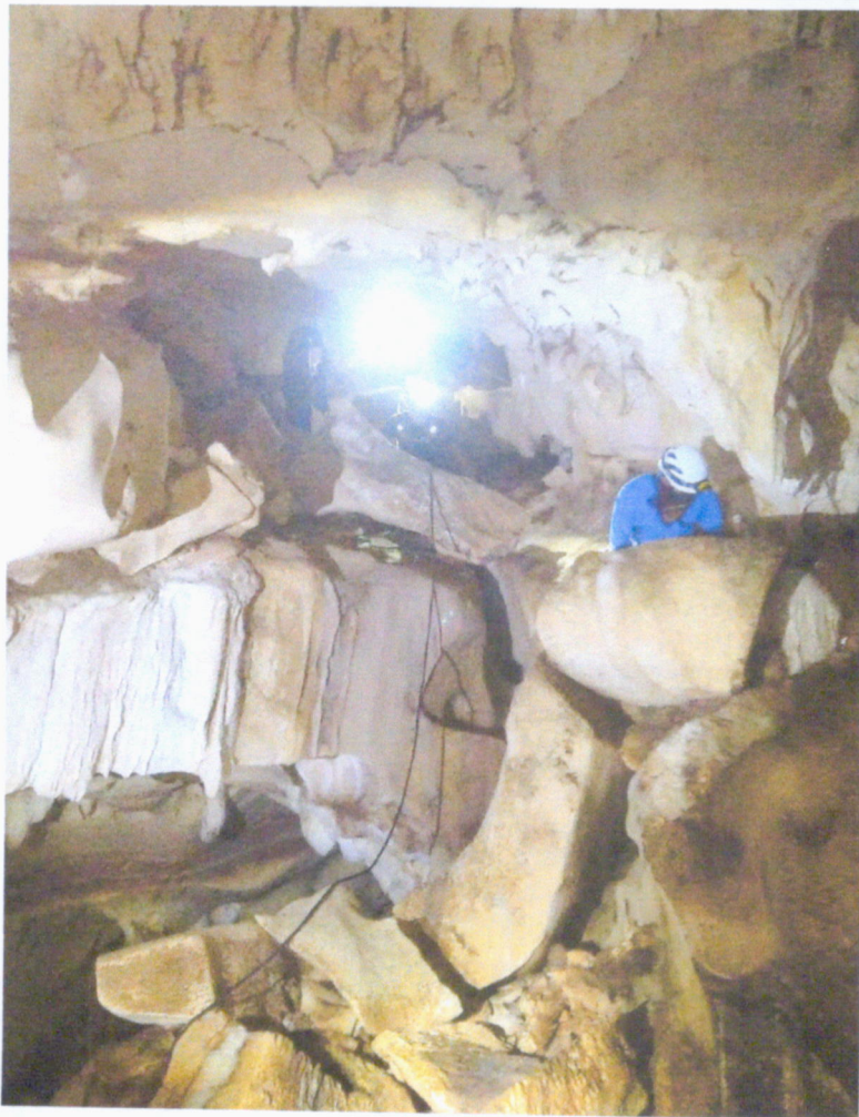
The team during the measurement of angle, orientation and distance between identified stations within the cave; in the photo are the tape 1 holder, clinometer and compass reader, and the recorder/cartographer
