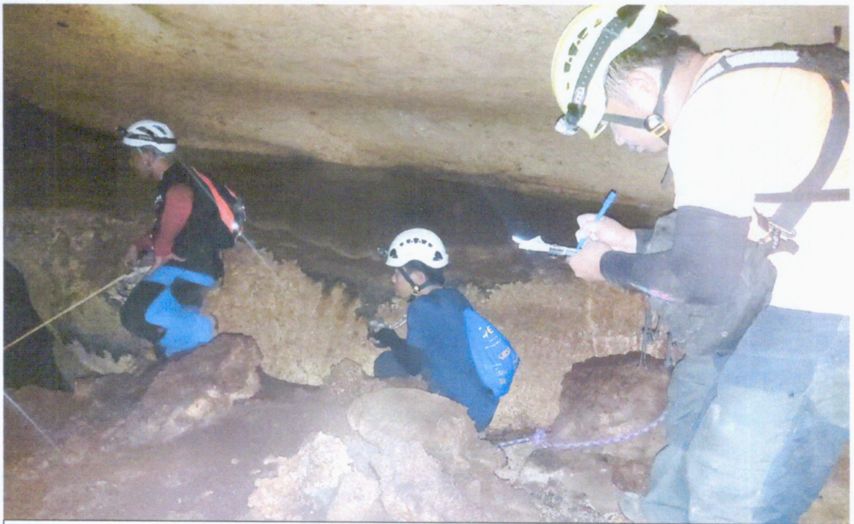
The team during the measurement of angle, orientation and distance between identified stations within the cave; in the photo are the tape 1 holder, clinometer and compass reader, and the recorder/cartographer
