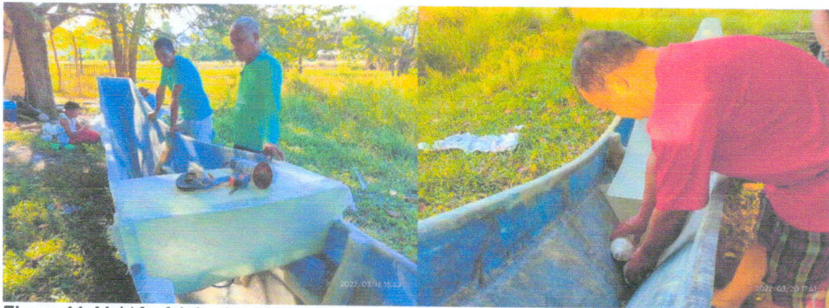
Figure 11. Mold for fabrication of fiberglass boat (left); Mr. Gammad shows how floaters (styrofoam inside pet bottles) are piled in the boat that helps on achieving buoyancy of the boat (right)
