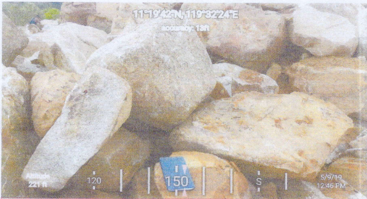
Photo No. 5: Boulder size rocks extracted from the adjacent hill, used as a basement filling material for the reclamation. Notebook as a scale
