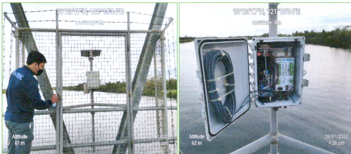
Figures 12: Pictures showing the spraying of WD40 to the lock of the gate (left) and the inside of the data logger of the Automated Water Level Station with no damage during the time of monitoring
