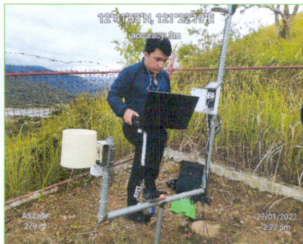
Figures 2: Photos showing the manual updating of the firmware of data logger thru the use of a laptop with updated Zentra Utility app.
