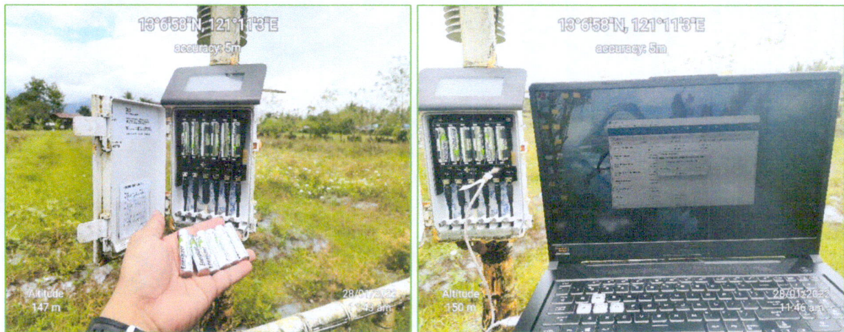
Figures 6: Pictures showing the rechargeable batteries for replacement to the old ones and the manual updating of the firmware of the data logger of the AWS
