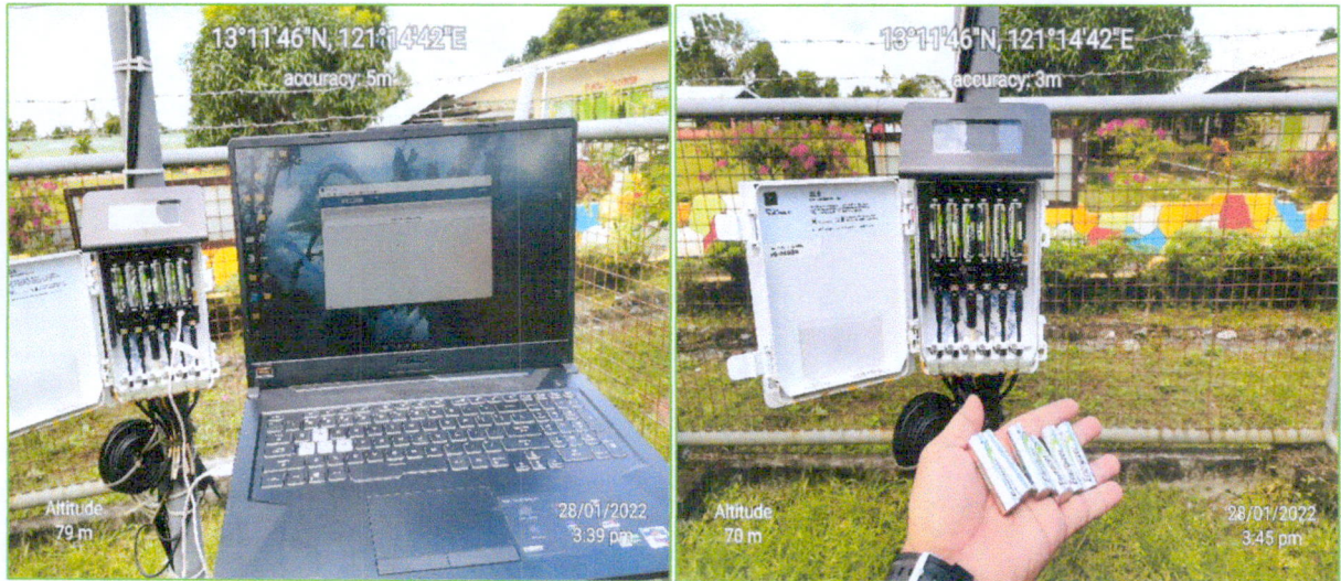
Figures 10: Pictures showing the rechargeable batteries for replacement to the old ones and the manual updating of the firmware of the data logger of the AWS
