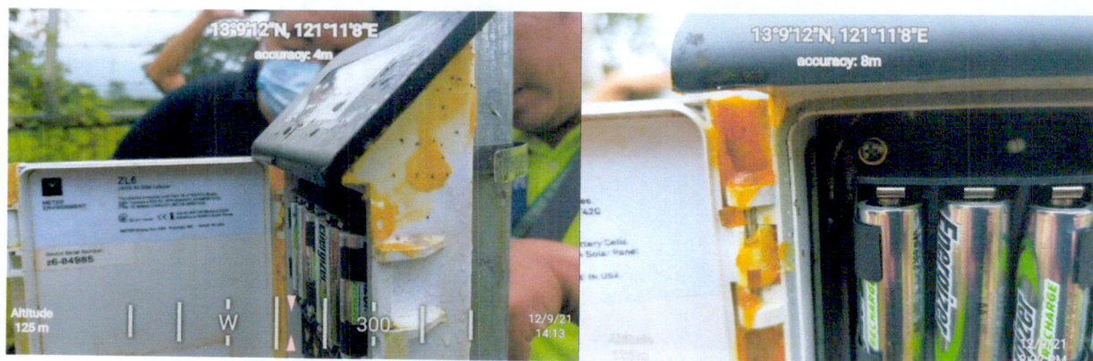
Fig. 3. Ant infestation in the datalogger of GWMS.
