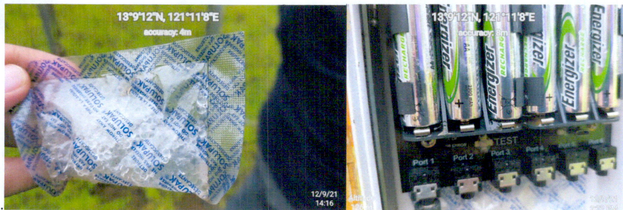
Fig. 2. Rainwater-soaked dessicant (right) and batteries (left) inside the datalogger of GWMS.
