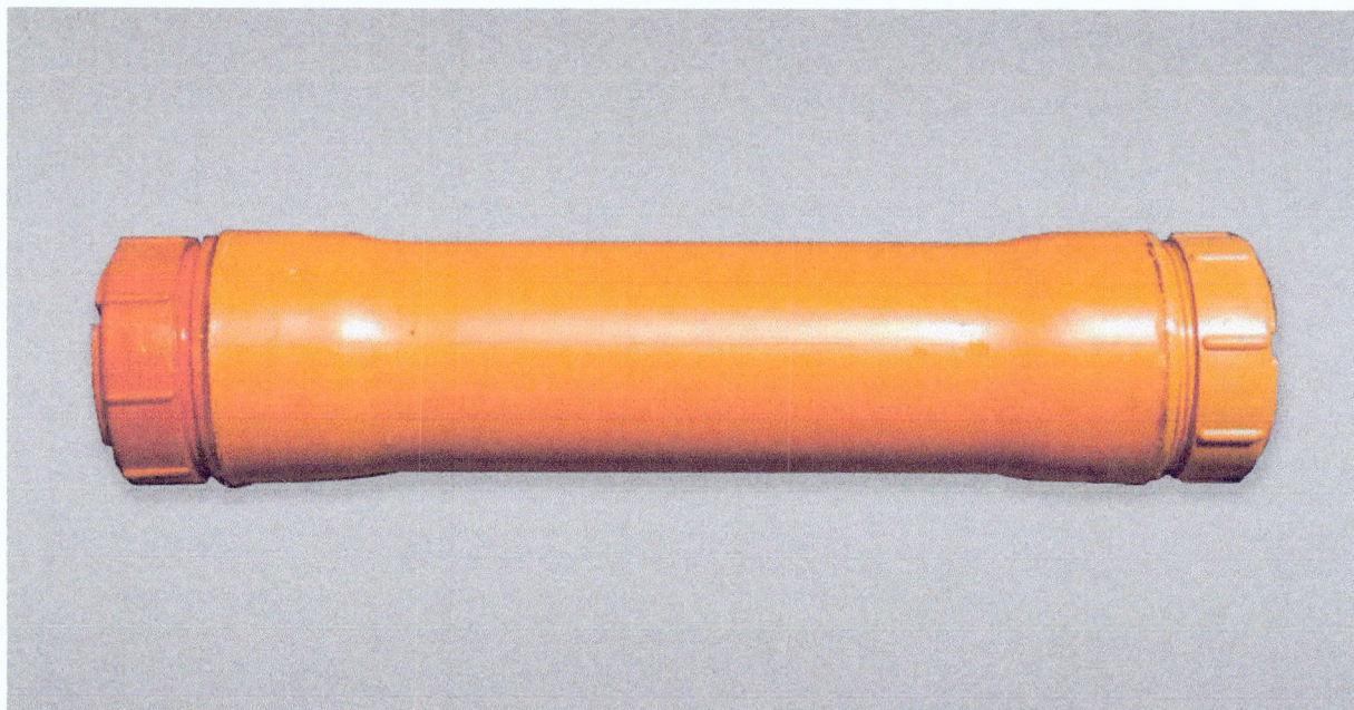
Figure 2. PVC sampling device used in collecting samples from different depths (surface, middle-layer, and near-bottom) at Ego Wall.
