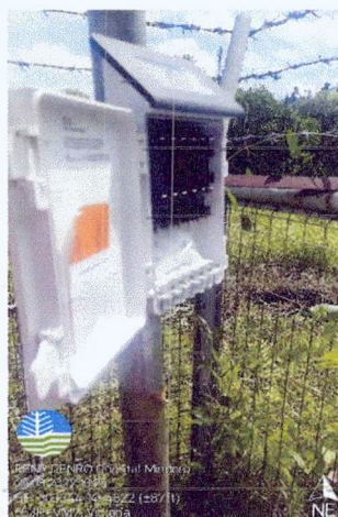
Installation of newly purchased ZL6 Data Logger for Ground Water Level Monitoring Station at MinSU Compound, Victoria, Oriental Mindoro
