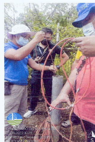
Installation of newly purchased ZL6 Data Logger for Ground Water Level Monitoring Station at MinSU Compound, Victoria, Oriental Mindoro
