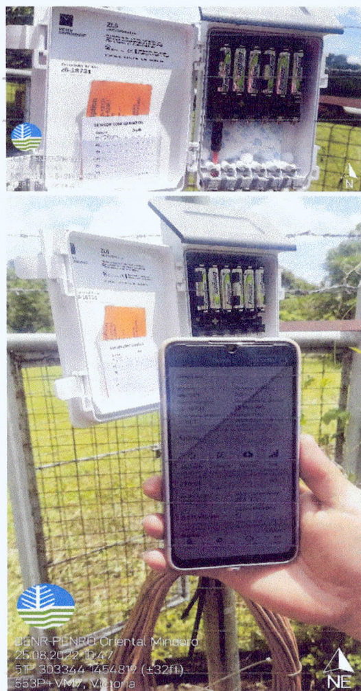
Installation of newly purchased ZL6 Data Logger for Ground Water Level Monitoring Station at MinSU Compound, Victoria, Oriental Mindoro
