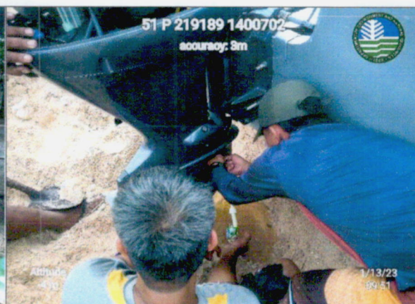
Boat Captain Mark Dennis Barretto and Park Maintenance Foreman Roberto Beringuela changing the oil of the 30-footer hi-speed watercraft
