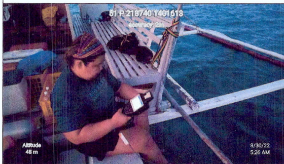
PASu Krystal Dayne T. Villanada measuring several parameters in-situ with a Horiba U-50 Multiparameter Water Quality Checker
