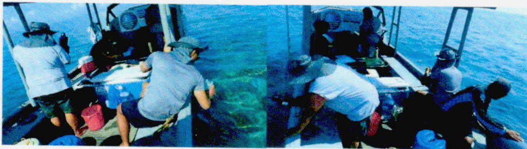
Figure 1. In situ collection of water parameters using the Horiba U50 and collection of water samples using grab sampling. Marine park rangers assisted TMO researchers in collecting water samples.
