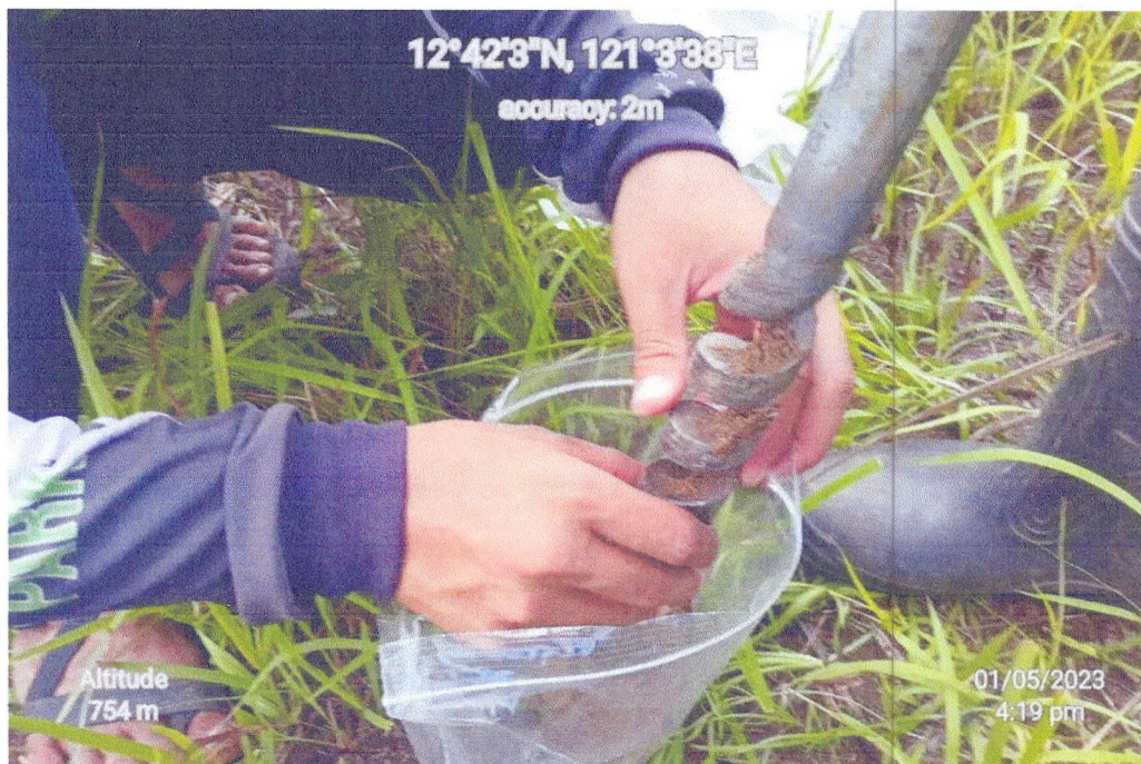
Figure 1. Soil sample taken at the MIBNP using a soil auger.
