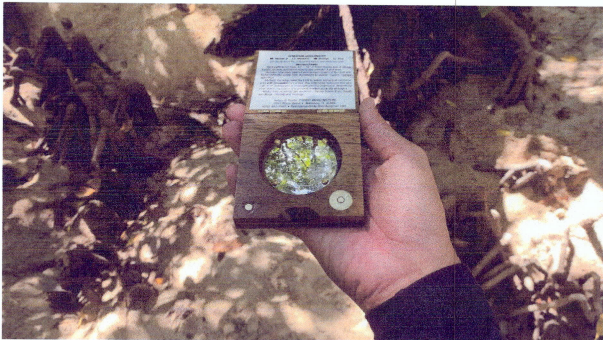
Figure 2. Convex spherical densiometer used in measuring canopy cover in the mangrove forest monitoring plots.
