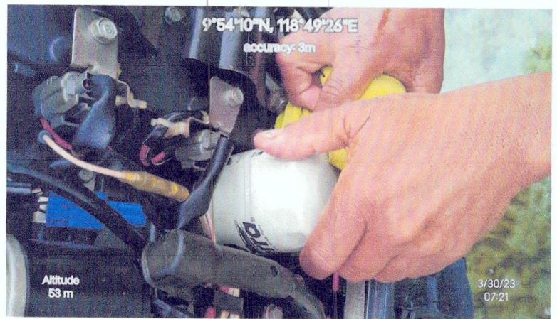
Photos during change oil and oil filter change of Snake Island speedboat on March 30, 2023
