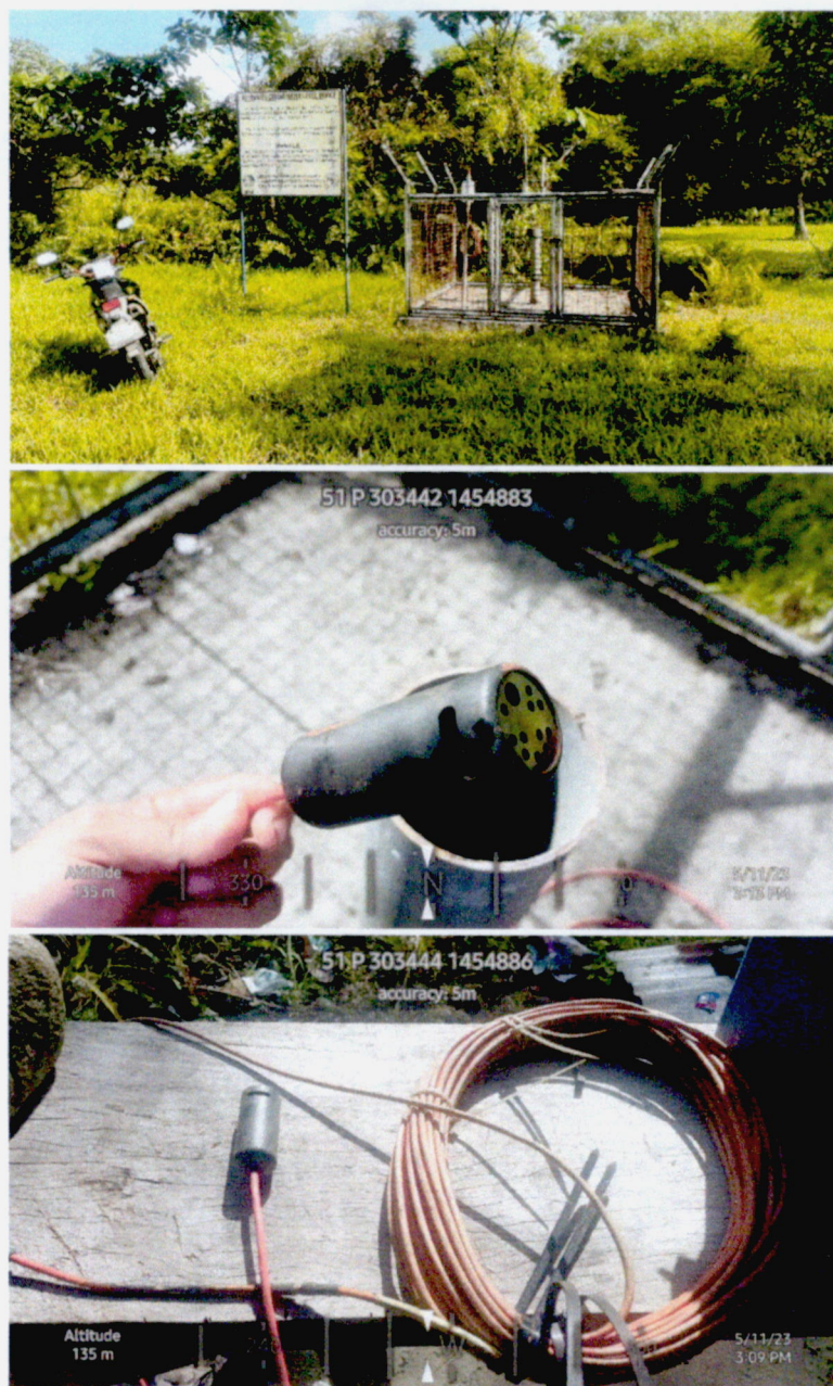
Figure 5. The MinSU-CTD (GWMS) station cleaning of CTD sensor and site monitoring on May 11, 2023.
